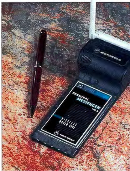
Motorola's Personal Messenger 100D is a wireless modem with all its components packed into a single PC Card.
