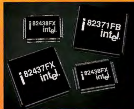
The Triton chip set supports bus mastering, EDO memory, and native signal processing.
