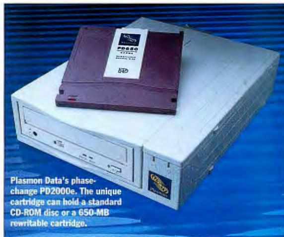
Plasmon Data's phase-change PD2000e. The unique cartridge can hold a standard CD-ROM disc or a 650-MB rewritable cartridge.
