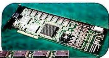
The Glint accelerator is the first chip to support the Internet 3-D graphics standard called Virtual Reality Modeling Language (VRML), which integrates 3-D viewing, navigating, and browsing on
