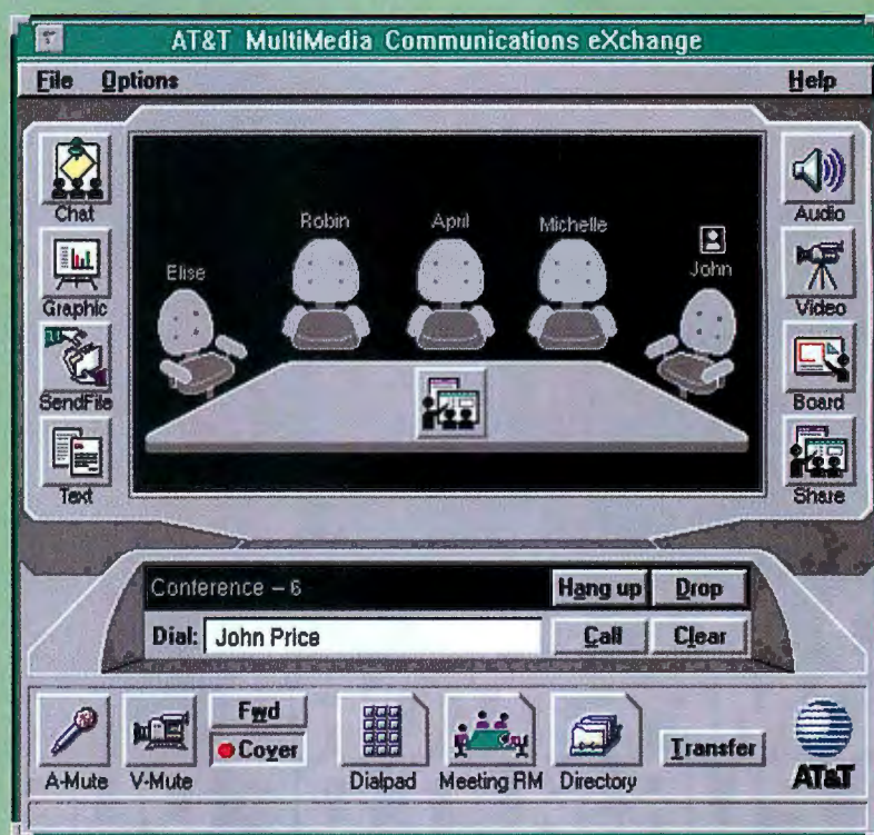
With AT&T's Multimedia Communications Exchange Server (MMCX), team members can get together in a virtual "meeting room." Along with providing a visual representation of the virtual meeting, MMCX combines multimedia calling features with collaboration tools to allow users to add or drop services and media as they choose.
