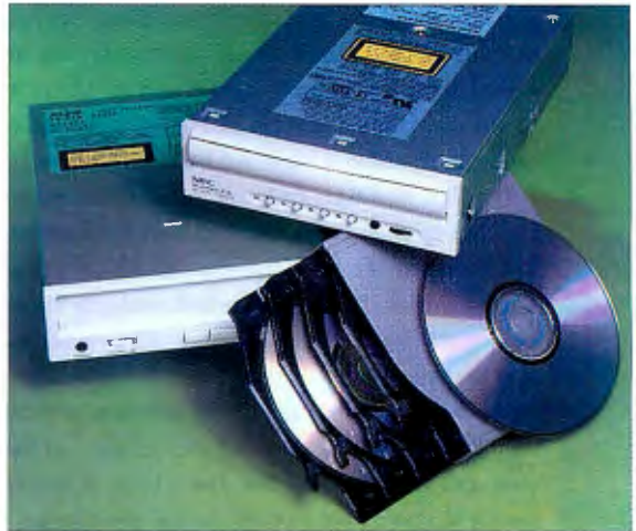
Both the Alps 4X (bottom) and the NEC MultiSpin pack four discs into a half-height 5¼-inch form factor. The Alps unit uses a cartridge (shown), while the NEC drive feeds in bare discs. Other similarities are quad speed (600 KBps) and an EIDE interface (adapter card included).
