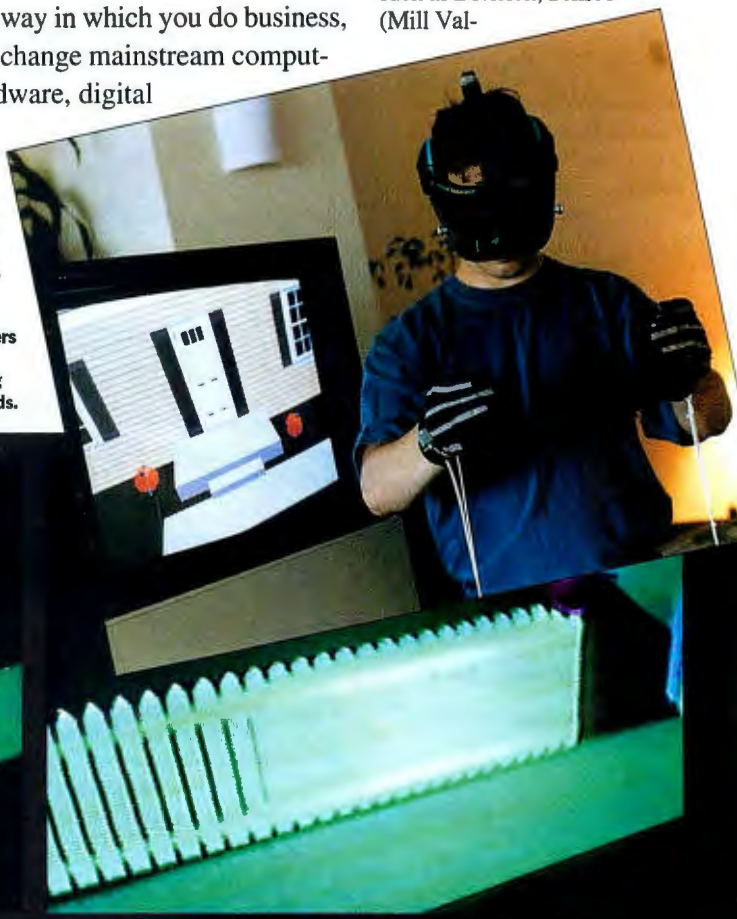
MultiGen's toolkit lets you stretch and manipulate objects. Here the designer is stretching the picket fence to cordon off a lawn.
