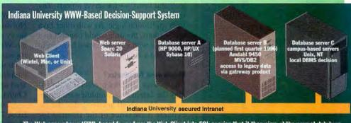
The Web server turns HTML-based forms from the Web Client into SQL queries that it then aims at the correct database server. The Web server formats the data returning from the database. The Web client browser calls up appropriate "viewers" (e.g., spreadsheets).
