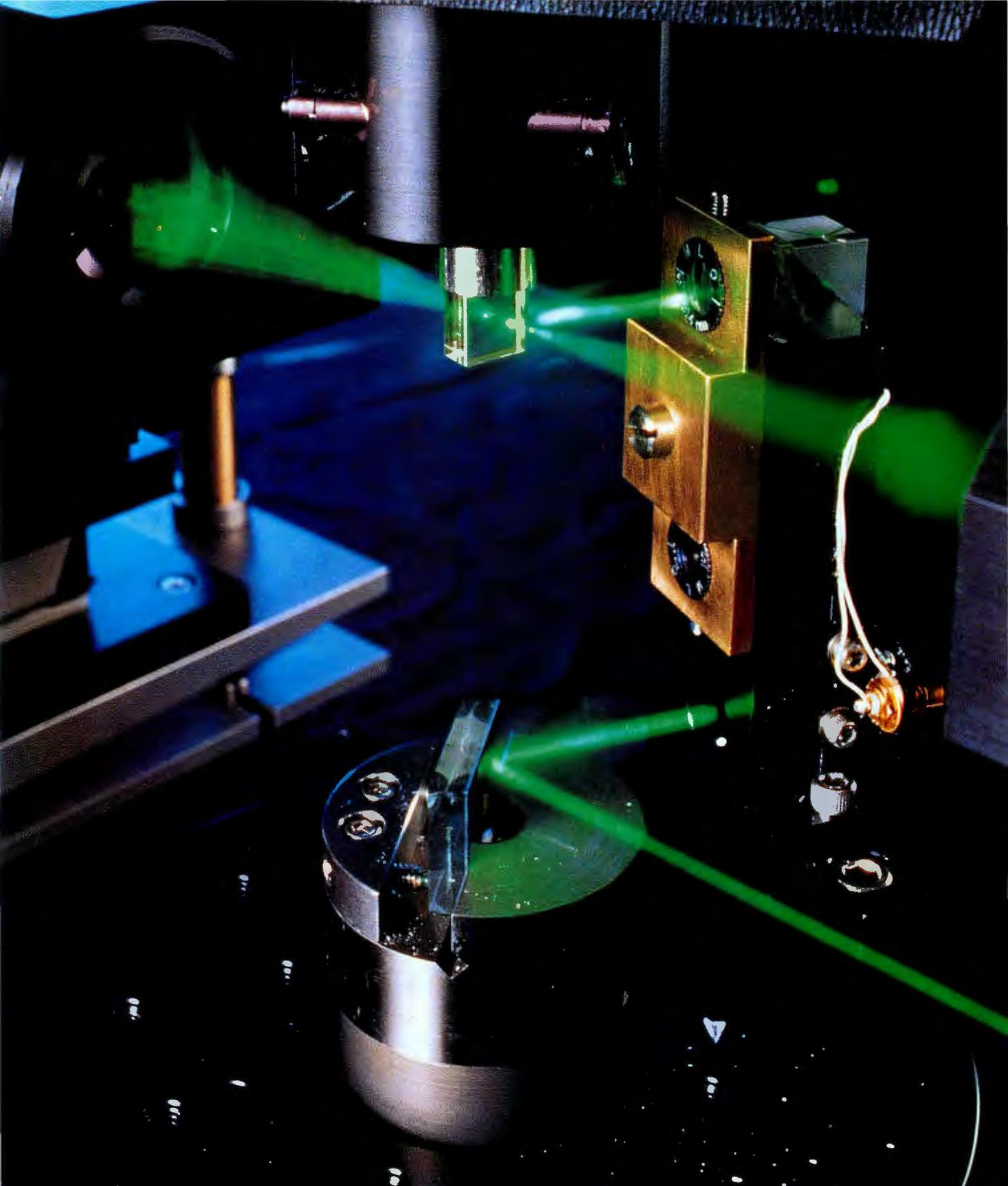
Future mass-storage devices might use holograms to record digital information on a doped crystal, in a way similar to that of the test apparatus shown here at IBM's Almaden Research Center. Commercial-scale equipment would be much smaller, have no moving parts, and use a high-powered semiconductor red laser. A crystal the size of a pack of playing cards would hold a terabyte of data.
