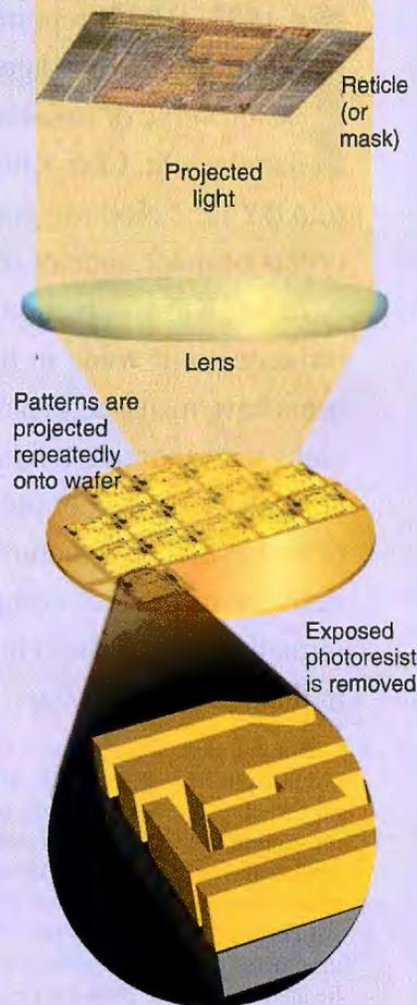
Chip vendors use photolithography to etch patterns onto doped silicon layers. The smallness of the features is limited by the frequency of the light beam and the resolution of the lens.
