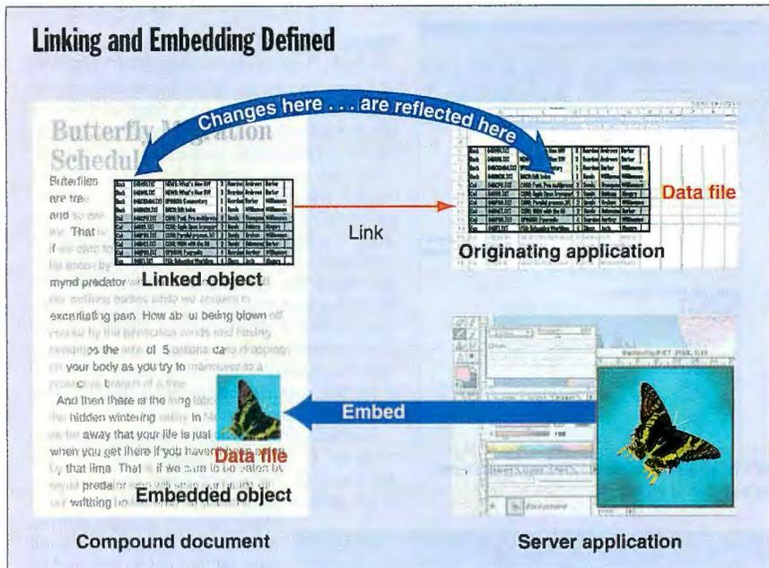
At bottom, most OLE 2 functions involve either linking or embedding. Linking maintains a connection only from the linked object to the application in which it was created. Embedding transfers and translates the server application's data so it can be independently stored in the compound document. Drag-and-drop and clipboard transfers are fundamentally embedding operations.
