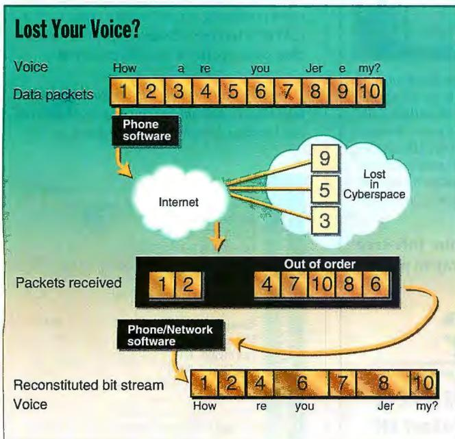
A much simplified depiction of what happens when speech is converted into digital packets that are sent through a network and received out of order, with pieces missing. Since the original was created in real time, a missing packet can't be resent, thus creating a gap in the data stream, which the recipient hears as clipped words or run-together speech.
