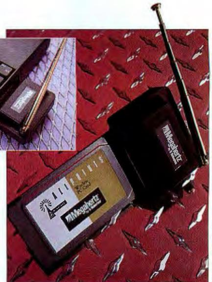
The Megahertz AllPoints radio modem looks like a PC Card wearing a backpack radio, with its attached 9-V battery module and 6-inch telescoping antenna.
