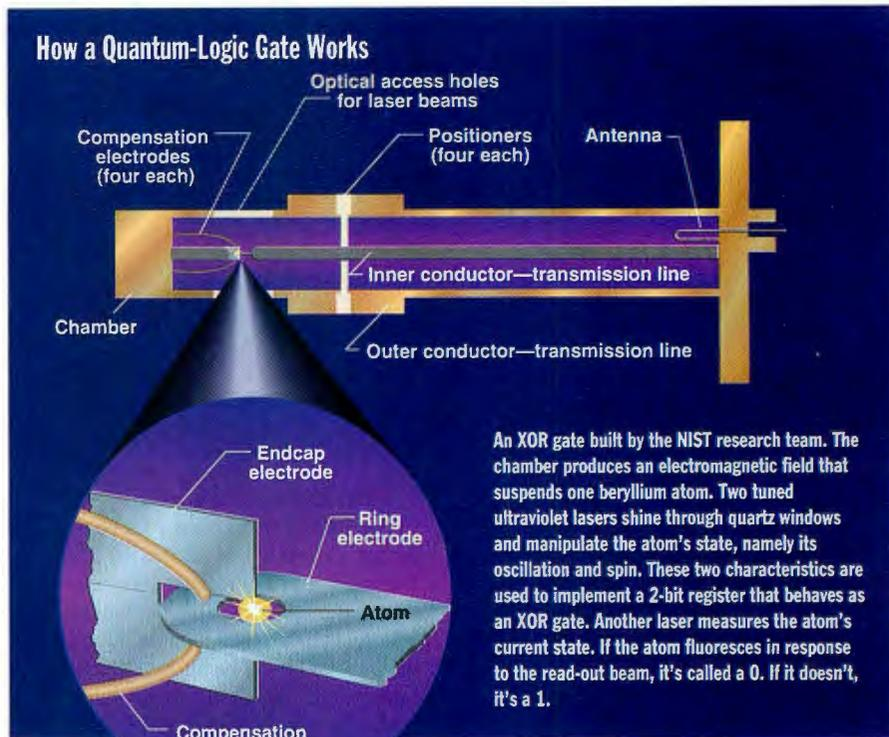
An XOR gate built by the NIST research team. The chamber produces an electromagnetic field that suspends one beryllium atom. Two tuned ultraviolet lasers shine through quartz windows and manipulate the atom's state, namely its oscillation and spin. These two characteristics are used to implement a 2-bit register that behaves as an XOR gate. Another laser measures the atom's current state. If the atom fluoresces in response to the read-out beam, it's called a 0. If it doesn't, it's a 1.
