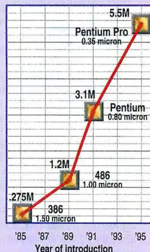
The x86 processor's transistor count has increased by 20 times in 10 years.
