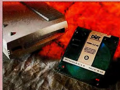
Using a single-write-pass technology, Pinnacle Micro's Apex 4.6GB rewritable magneto-optical drive offers near-hard-drive performance and has a low per-megabyte cost.
