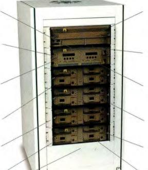
Optional Sphinx unit to rackmount a desktop SPARC®, HP or SGI workstation for network addressable RAID.
