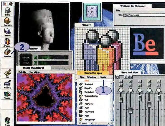
The multitasking, multithreaded Be OS automatically assigns each window two threads. In addition, every object is stored in a built-in relational database, with its attributes (1). You can query the database on any attribute (2).
