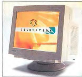
dows 95, and VESA's new communications standard for the Display Data Channel. The monitors include ultrahigh resolutions up to 1280 by 1024 pixels noninterlaced, refresh rates up to 75 Hz at 1024 by 768 pixels, and a super-fine 0.25mm aperture pitch.
