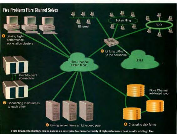
port "calls" the fabric by entering the address of the destination port in a frame header. The fabric does all the work of setting up the desired connection. The originator does not have to worry about complex routing algorithms, and there are no complicated Permanent Virtual Circuits (PVCs) to set up.
