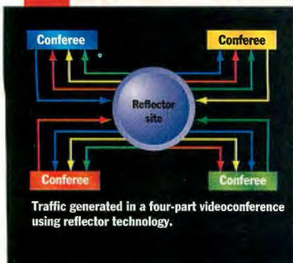
A reflector cuts the data each conferee must transmit on a point-to-point network.
