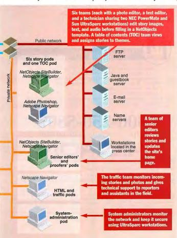
so they prepared for the worst. MFS Communications hooked the Cyber24 site directly into its prime Internet hubs on the Atlantic and Pacific coasts. These hubs, known as Metro Area Exchange (MAE) East and MAE West, are the gateways to a high-speed fiber-optic backbone that uses asynchronous transfer mode (ATM) and synchronous optical network (SONET). DS-3 and T1 lines connected project servers to the hubs.
