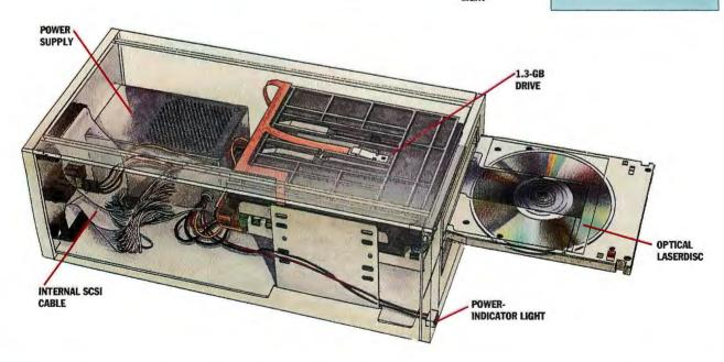
means of data storage, as they aren't affected by magnetic fields. This technology will let drives like Panasonic's support the emerging high-density digital videodisc (DVD) CD-ROM format for the entertainment industry.
