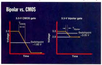
Bipolar transistors are inherently faster than CMOS transistors, partly because CMOS transistors must swing from their highest voltage to their lowest voltage to change states. Bipolar transistors swing between intermediate voltages. However, bipolar runs very hot. Exponential's chip may dissipate 40 to 60 W, compared to about 20 W for a 400-MHz Alpha 21164.
