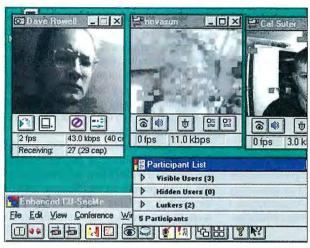
Connectix VideoPhone (Windows version at left) doesn't vet work across platforms but provides better imaging and more professional features than does Enhanced CU-SeeMe (below). Only the Mac version of VideoPhone supports multiperson conferencing. It uses multicasting. while CU-SeeMe requires reflector sites. All these programs require significant network bandwidth for any quality at all. With a 28.8-Kbps modem hookup, the frame rate often falls below one per second.
