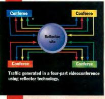
A reflector cuts the data each conferee must transmit on a point-to-point network.
