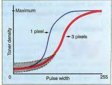
The relationship between toner density and laser pulse width doesn't allow for fine-tuning with single-pixel color dots. Using three-pixel color dots provides more range for control but suffers from noise variation at the low end.
