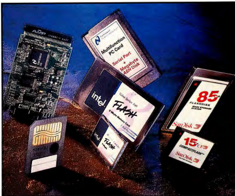
Flash-memory cards from Toshiba, National Semiconductor, Intel, or SanDisk can give up to 85 MB of solid-state storage—at $20 per MB.
