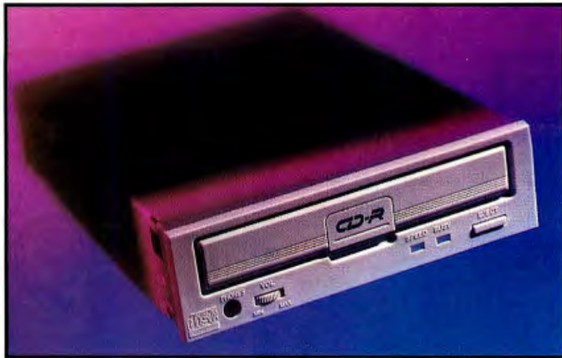
JVC's Personal RomMaker internal CD-R drive records and plays CDs at speeds of up to 4X.
