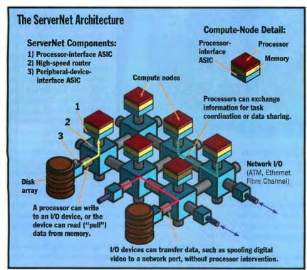
ers have multiple interconnections to processor nodes and devices, a ServerNet SAN can deliver spectacular performance. Tandem claims that a system with 4096 compute nodes and peripherals—and with 4680 to 7680 routers arranged in a fractahedral topology—can achieve an aggregate switching bandwidth of 410 GBps. By comparison, some supercomputers have a maximum switching bandwidth of only 1.2 to 2 GBps. (To be fair, these supercomputers achieve this rate with only 32 processors, not 4096.)
