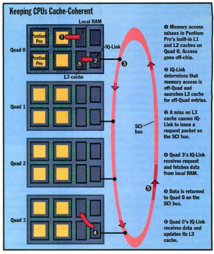
each SMP node runs its own copy of the OS and applications while sharing disks and communications peripherals with other nodes. Since each Quad has a PCI interface, you can distribute peripherals throughout the system to reduce competition for I/O devices. You have a choice of two OSes: DYNIX/ptx (Sequent's SMP-enhanced Unix) or Windows NT.
