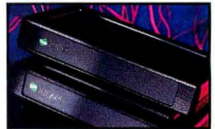
external solution with an ISA-based add-in card that you install inside your LAN server connected to an external box that has eight serial-port connections for external modems. This direct-to-LAN-server attachment may be cost-effective, but it takes its toll on your server.
