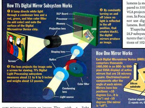
uses mirrors to create an image. The result of TI's Digital Light Processing (DLP) subsystem—now appearing in new PC projection systems—is bright, crisp output that's also visible from side viewing angles. And perhaps by this time next year, TI will have similar subsystems for high-quality color printers. The DLP technology is being used by In Focus Systems (Wilsonville, OR, 503-685-8888), Proxima (San Diego, CA, 619-457-5500), Nview (Newport News, VA, 804-873-
