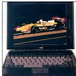
810-MB hard drive; a 3½-inch removable floppy drive; two Type II or one Type III PC Card slot; an 88-key keyboard with Windows 95 function keys; a touchpad pointing device; a 10.4- or 11.3-inch DSTN or TFT SVGA color display; a dual NiMH detachable/rechargeable battery supply; an AC power adapter; and Windows 95. Multimedia features include a quad-speed CD-ROM drive; two stereo speakers; 3-D sound and Sound Blaster Pro 16-compatible MPEG support; a microphone; and audio ports.
