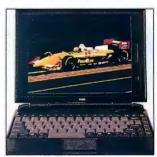
810-MB hard drive; a 31/2-inch removable floppy drive; two Type II or one Type III PC Card slot; an 88kev keyboard with Windows 95 function keys; a touchpad pointing device; a 10.4- or 11.3-inch DSTN or TFT SVGA color display; a dual NiMH detachable/rechargeable battery supply; an AC power adapter; and Windows 95. Multimedia features include a quadspeed CD-ROM drive; two stereo speakers; 3-D sound and Sound Blaster Pro 16-compatible MPEG support; a microphone; and audio ports.
