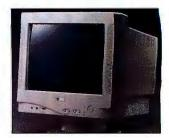
headset sockets built into the front of the bezel. The MM6536SL multimedia color monitor (\$445) features a horizontal frequency of 30 to 64 kHz, a vertical refresh rate of 50 to 100 Hz, a 1280- by 1024-pixel noninterlaced resolution, and a 0.28-mm dot pitch. The flat-square CRT has an enhanced nonglare, antistatic coating and an Invar shadow mask.
