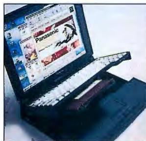
The CF-62 system comes with a 100- or 133-MHz Pentium CPU with 256 KB of L2 cache, 32-bit PCI bus architecture, 8 or 16 MB of EDO memory (expandable to 48 MB), a 12.1-inch 1024-by-768-pixel XGA or 800 by 600 SVGA color LCD, up to 1.35 GB of disk storage, a GlidePoint touchpad, a Chips &
