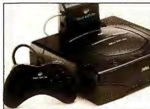
peripheral for the Sega Saturn, brings the Internet to your TV for networked gaming, e-mail, on-line chats, and Web connections. The modem plugs into the cartridge slot on the Sega Saturn, and the package has CD-ROM-based HTML 2.0-compatible Web-browser software developed specifically for the NTSC display standard.
