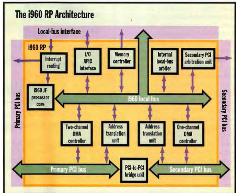
This intelligent I/O controller manages DMA transfers and memory timing. It also acts as a PCI-to-PCI bridge.
