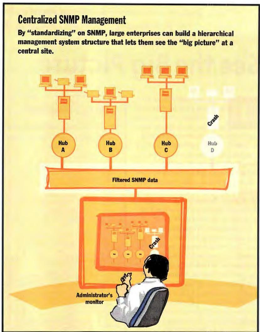
ety of SNMP-compliant devices and systems. This provides a broader view of the topology and status of the entire network (see the figure above). Most smaller networks do not require SNMP because they don't have the wide variety of hardware and software required in big networks.
