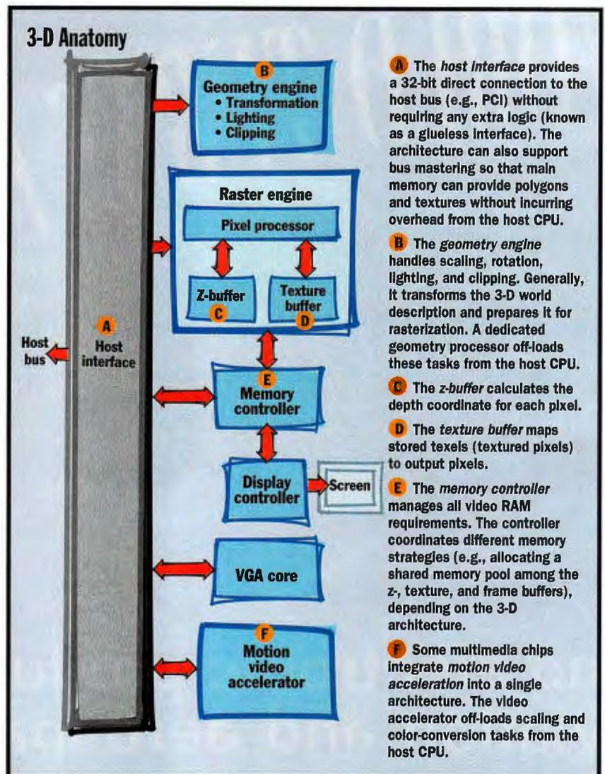
that's on a separate PCI board. After the 3-D chip calculates the pixels, they pass across the PCI bus to the graphics card.
