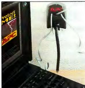
modem/fax lines—and a 6-foot telephone cord. A thermal fuse disconnects the AC line if there is a sustained overvoltage.
