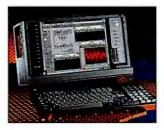
play, five full-size PCI/ISA expansion slots, a patented card-retention plate, and high-throughput cooling integrated in the 20-pound portable package. Complementing the dual 200-MHz Pentium Pro CPUs is system memory ranging from 8 to 768 MB and 256 or 512 KB (L2) of secondary cache memory. Available peripherals include CD-ROM drives, optical read/write drives, high-speed tape backup and floppy drives, and telecommunications and network cards for server applications.
