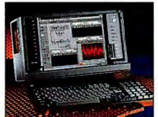
play, five full-size PCI/ISA expansion slots, a patented card-retention plate, and high-throughput cooling integrated in the 20-pound portable package. Complementing the dual 200-MHz Pentium Pro CPUs is system memory ranging from 8 to 768 MB and 256 or 512 KB (L2) of secondary cache memory. Available peripherals include CD-ROM drives, optical read/write drives, high-speed tape backup and floppy drives, and telecommunications and network cards for server applications.
