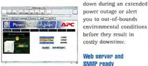
PowerChute plus provides unattended system shutdown and UPS management for Windows NT. Netware and other servers. Manage Smart-UPS via SNMP, DMI and Web browsers (shown above). Features vary by operating system.
