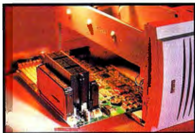
The swappable processor board easily snaps onto the motherboard.
