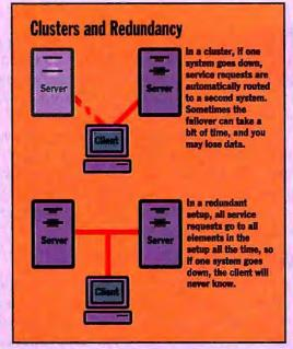
Clustering and redundant arrays of systems are two approaches to HA and FT.
