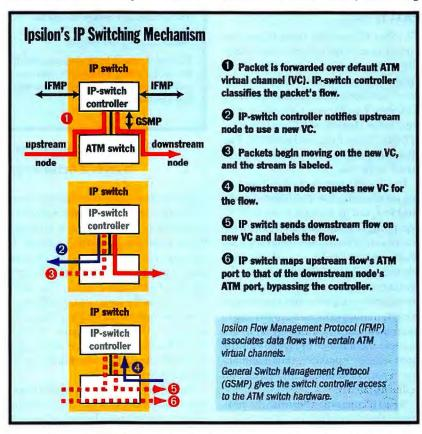
You can send low-latency data directly through an ATM virtual channel, bypassing the IP controllers.
