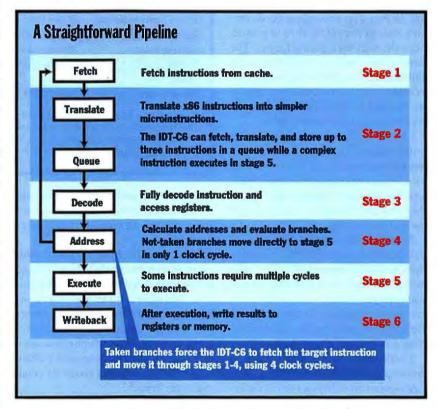
The IDT-C6's pipeline resembles a 486 pipeline.
