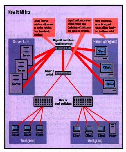
Gigabit Ethernet switches, routing switches, Layer 2 switches, hubs, and port switches can all play a part in a network architecture.
