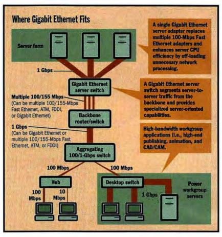
Gigabit Ethernet makes sense as a way of linking Fast Ethernet LANs with servers and each other.
