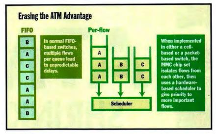
In MMC's Xstream chip set, packets and cells both gain from a scheduler that gives priority to time-sensitive traffic.
