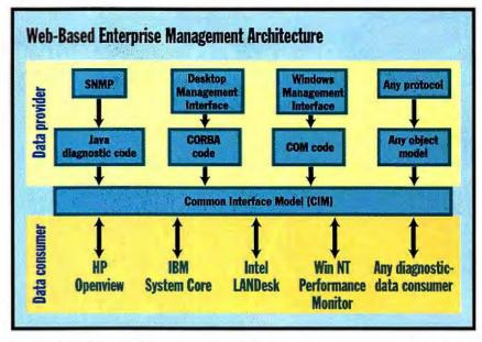
The WBEM architecture allows devices and management tools to send and retrieve diagnostic data, despite differences in protocols.
