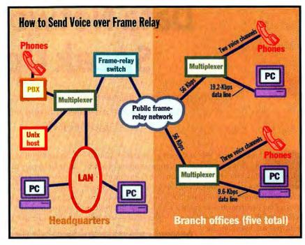
A Miami food distributor needed only to add multiplexers and switches to send voice over its data network and cut phone charges.
