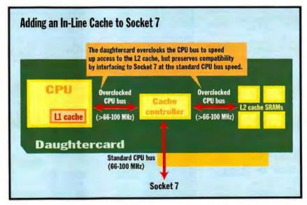
An in-line L2 cache doesn't require a backside bus, so it would work with existing processors.
