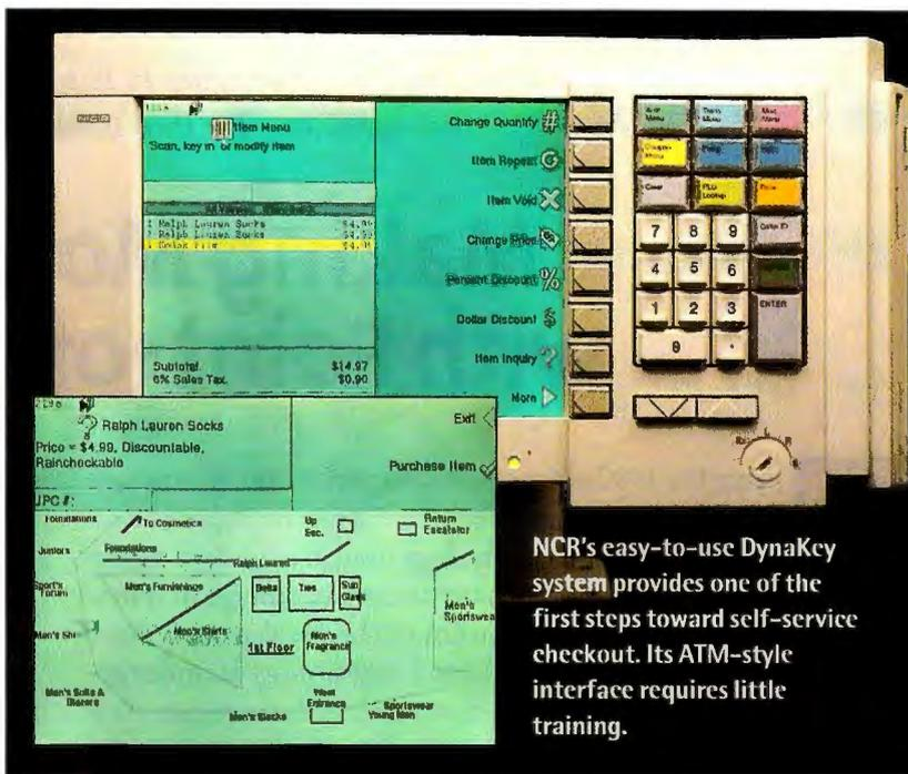
NCR's easy-to-use DynaKey system provides one of the first steps toward self-service checkout. Its ATM-style interface requires little training.
