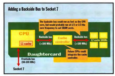
CPU designers could make a Socket 7-compatible backside bus by segregating the L2 cache on a daughtercard.
