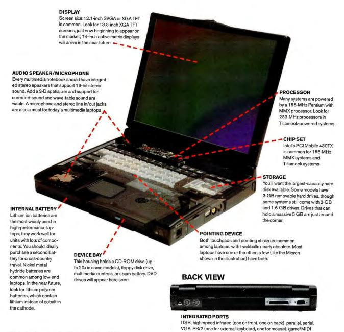
Illustration based on the Micron TransPort XKE.
