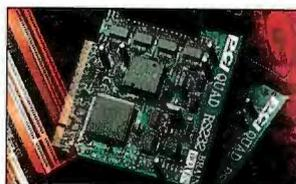
to 115.2 Kbps, includes a 16-byte FIFO buffer, and comes with software utilities for DOS and Windows 95, NT, and 3.11.
