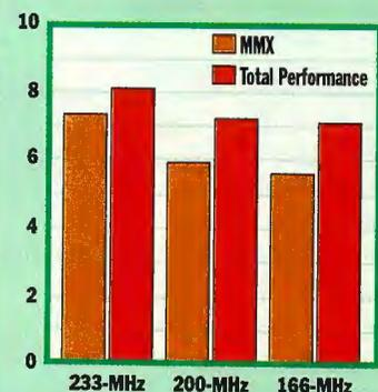
Average MMX scores (scaled 1-10) compared by CPU speed.
