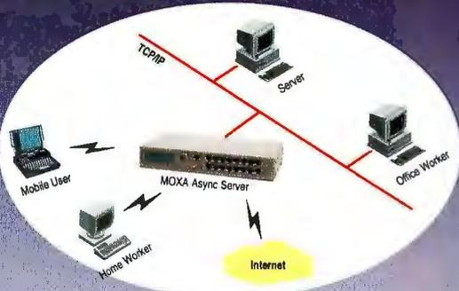
Remote Access environment allows remote users with access to corporate LAN resource or local users with connections to remote workgroups or Internet. MOXA Terminal Server and Multiport serial board provide you with the best and alternative solutions.
