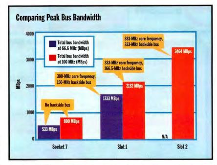
Intel's CPU slots offer more peak bus bandwidth than Socket 7 because they drive a backside bus at higher frequencies.
