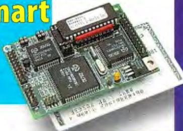
Z-World's powerful BL1500 controller is ideal for OEM machine control and data acquisition, especially when analog I/O is required.
