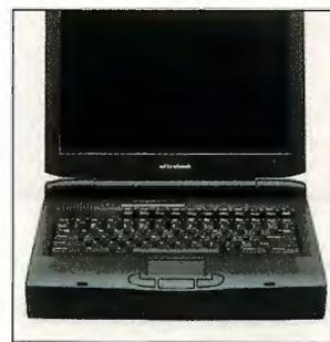
powered notebook has a 200-MHz UltraSPARC processor, a 14.1-inch active-matrix LCD, and a 9-GB EIDE hard drive for portable processing power. It includes 32 to 512 MB of memory and a PCI-based ATI Rage LT Sun Creator 2-D or 3-D graphics accelerator. The UltraBook runs unmodified Solaris 2.5.1 or 2.6 and is compatible with Sun Microsystems workstations.
