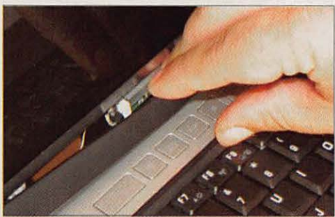
Once you've removed all of the bezel's securing screws, gently pull the bezel away from the LCD.
