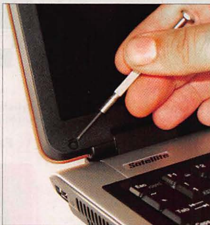
Carefully pry back the small rubber covers on the bezel to reveal the screws holding it in place.
