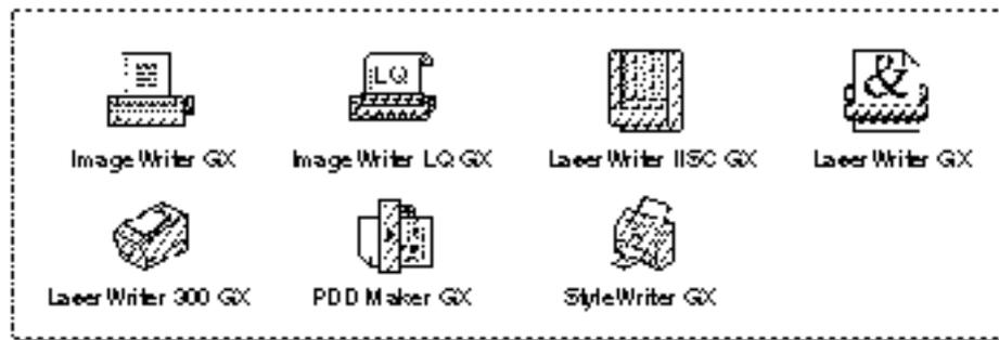
These devices need not represent actual physical devices on the system. In particular, the portable digital document printer driver, represented by the PDD Maker GX icon, is used only to create a document that is packaged ready-to-view on another computer.
