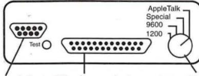
9-pin socket 25-pin socket 4-position mode switch
