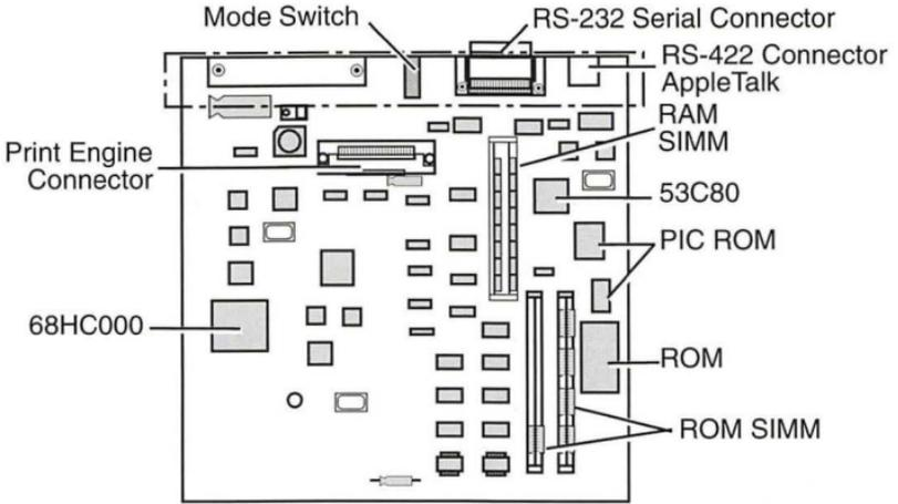
Figure: NT I/O Board
