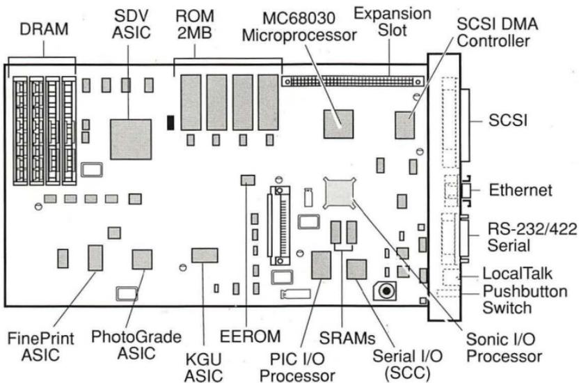
**Figure: Ilf Controller-I/O Board**
