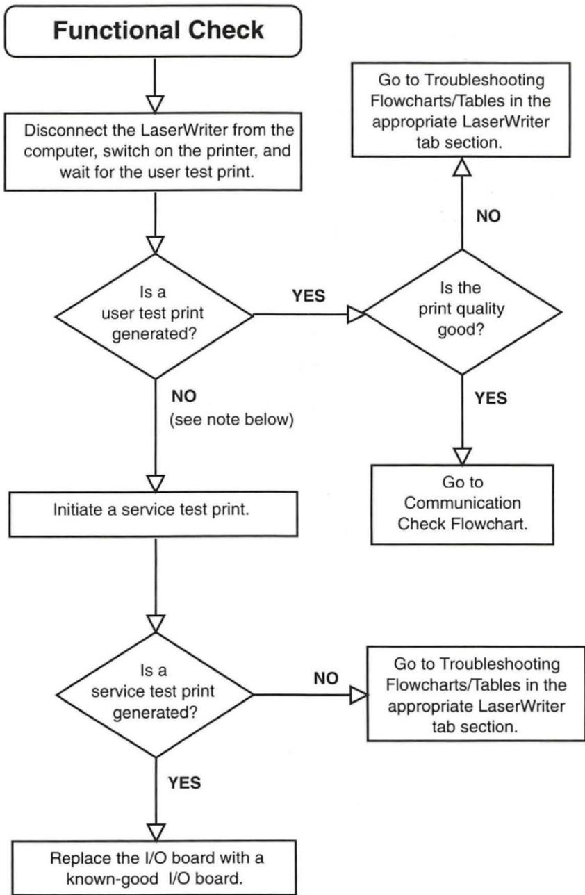
**Note:** The LaserWriter, LaserWriter II NT, NTX, II, IIG, and Personal LaserWriter NT produce a user test print each time the printer is switched on (unless the function has been turned off with PostScript software). The LaserWriter II SC and Personal LaserWriter SC produce a user test print only if the SCSI ID switch is set to "7." The Personal LaserWriter LS does not produce a user test print.
