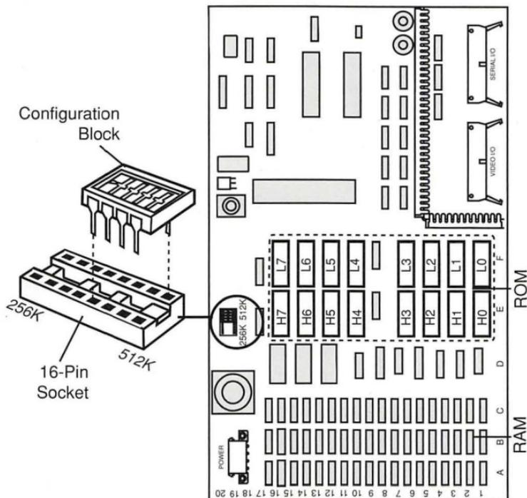
Figure: LaserWriter 256K/512K I/O Board
