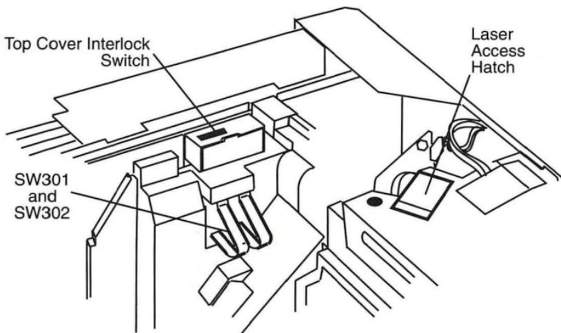
Figure: Laser Power Output Check Controls
