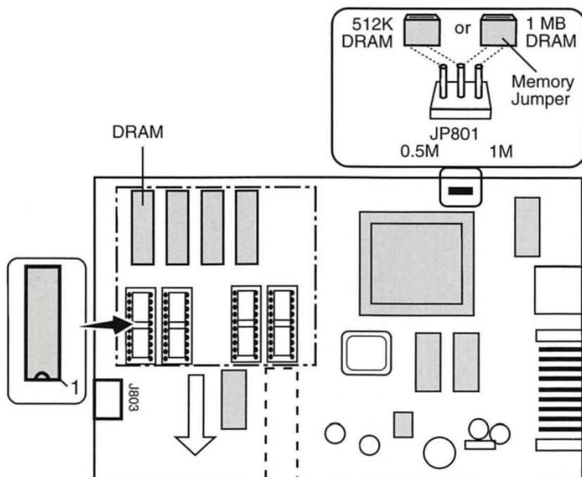
Figure: LaserWriter LS Memory Upgrade
