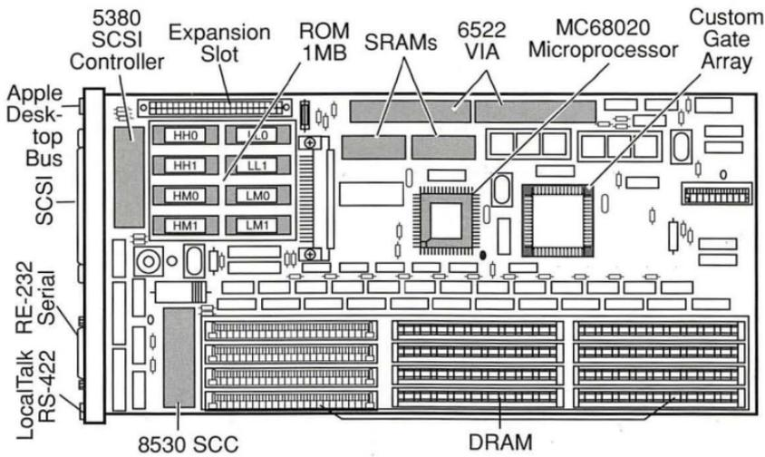
**Figure: NTX Controller-I/O Board**
