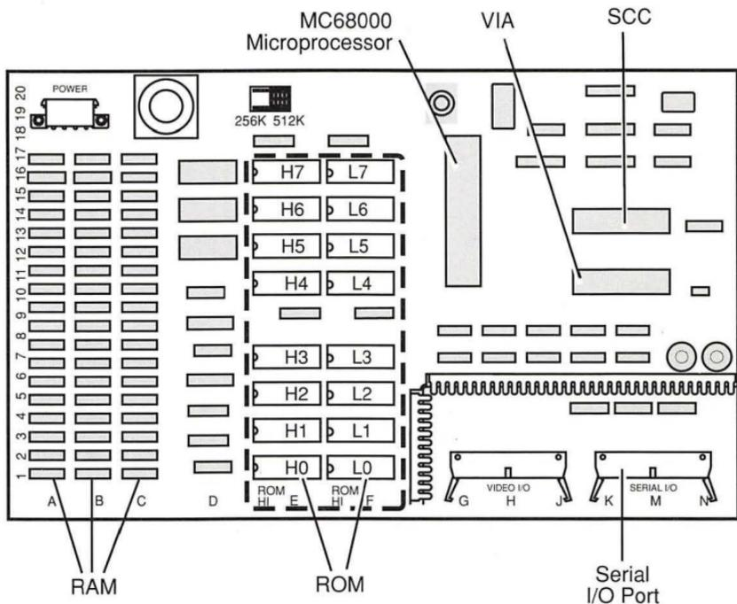
Figure: LaserWriter I/O Board
