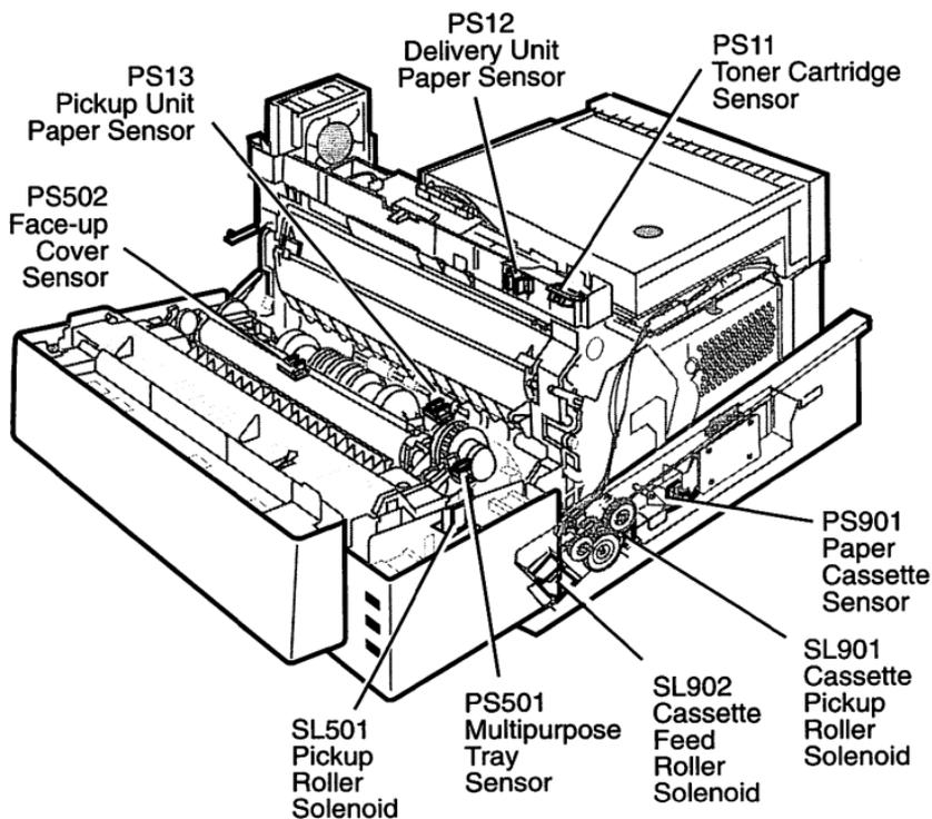
Figure: Sensors and Solenoids
