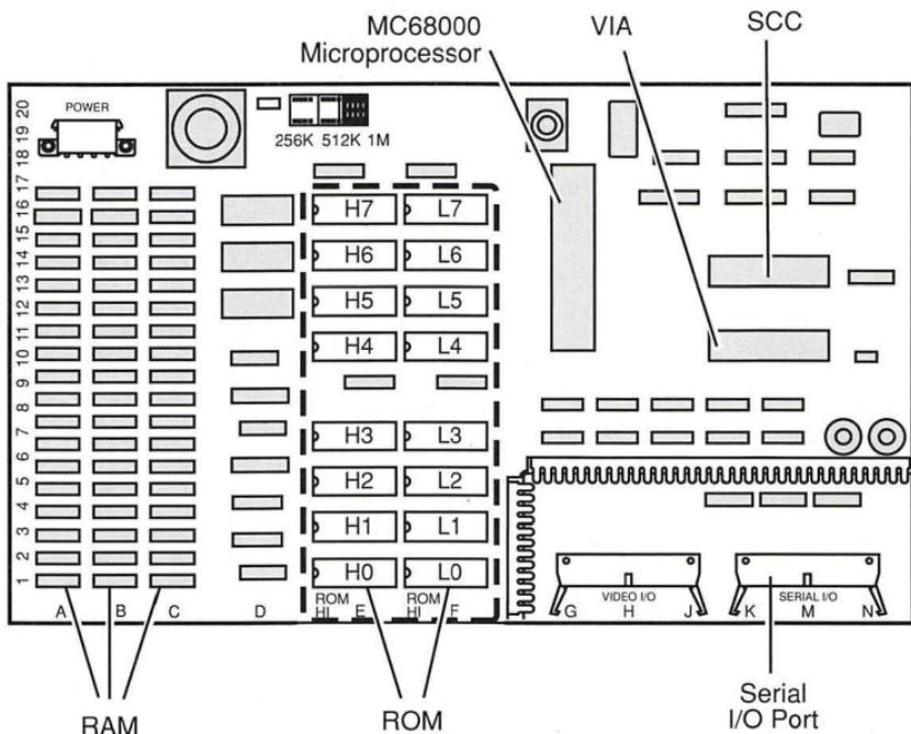
Figure: LaserWriter Plus I/O Board
