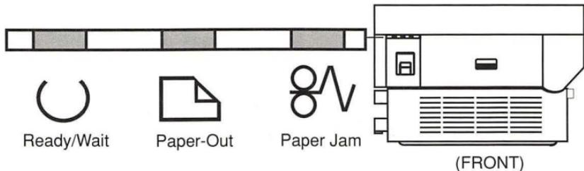
Figure: LaserWriter/LaserWriter Plus Status Lights
