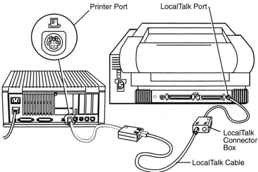
Figure: AppleTalk Connection
