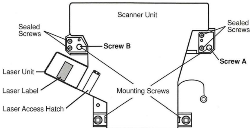
Figure: Laser/Scanner Unit
