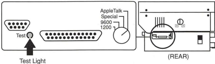
Figure: LaserWriter/LaserWriter Plus Test Light
