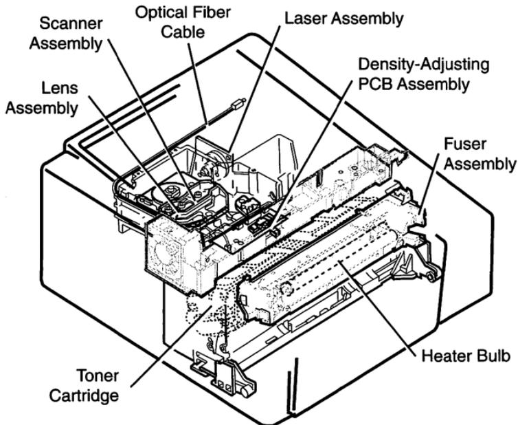
Figure: Internal Assembly Locations
