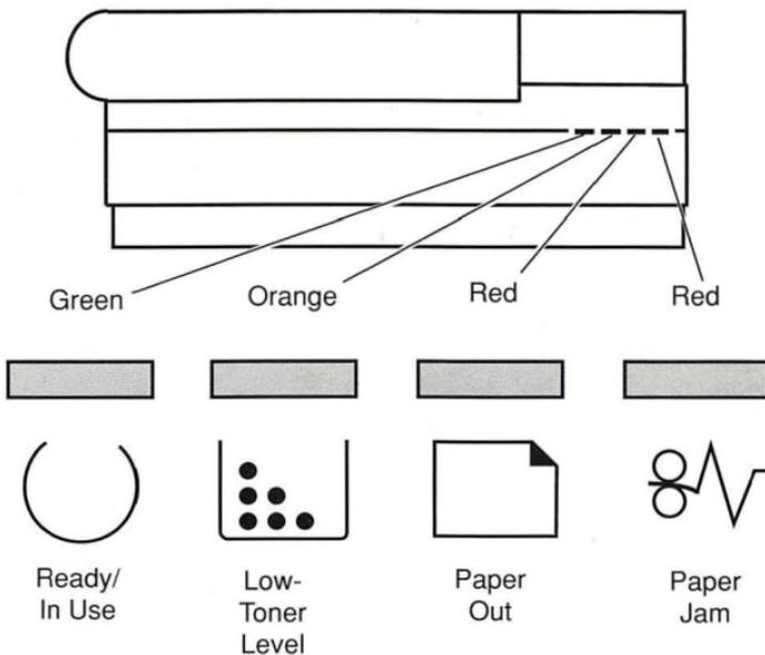
Figure: LaserWriter II Status LEDs
