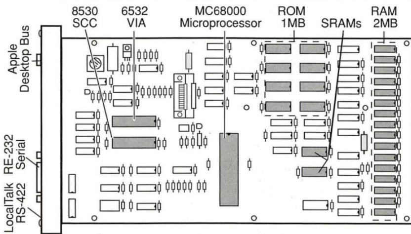
**Figure: NT Controller-I/O Board**
