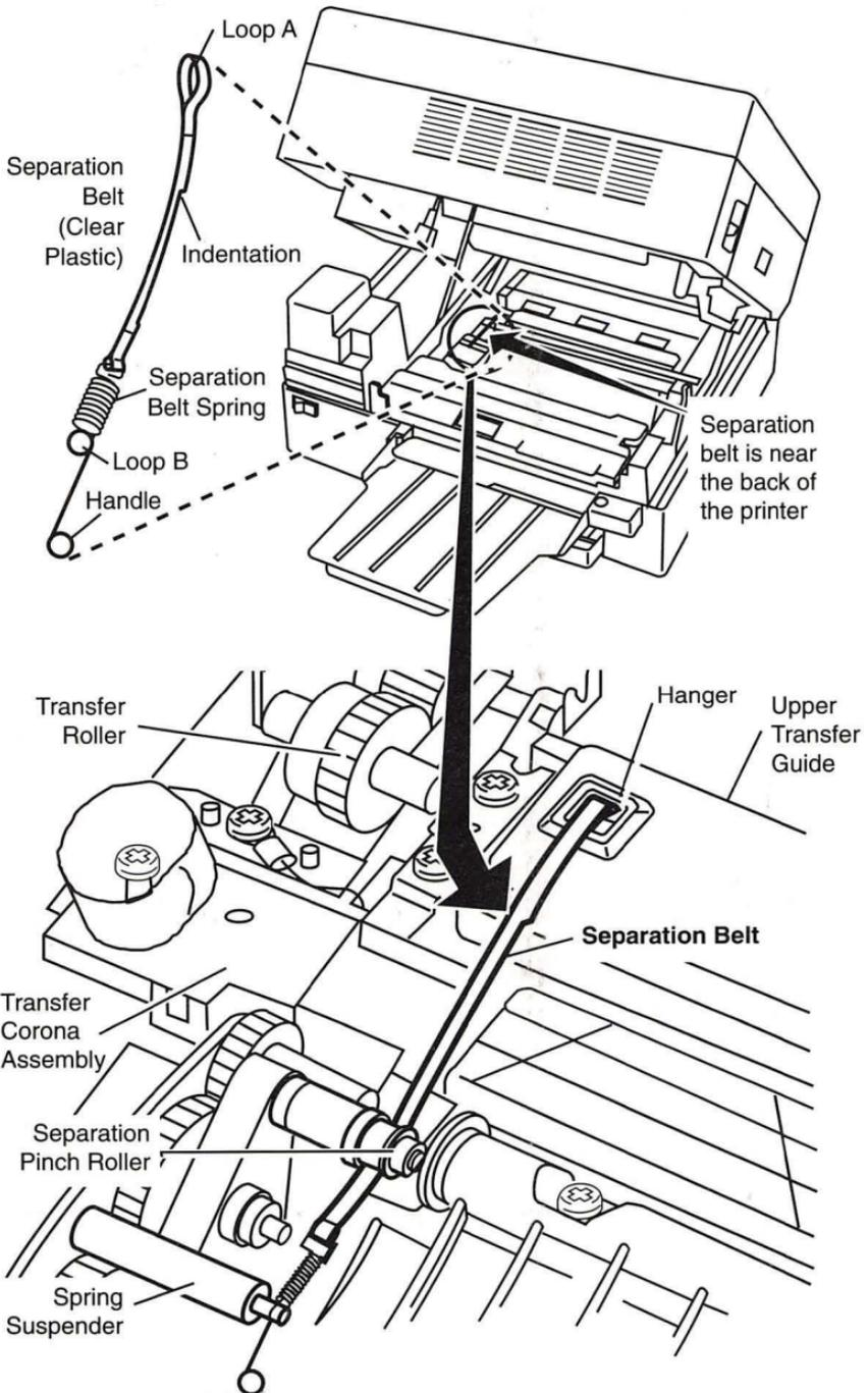
Figure: Installing the Separation Belt
