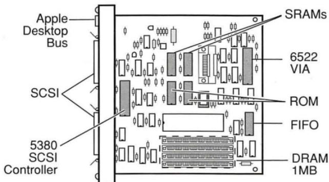
**Figure: SC Controller-I/O Board**
