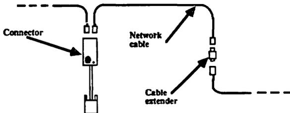
The AppleTalk connector is attached to a computer or other device; the individual AppleTalk connectors are then linked by means of the network cables. When all of the lengths of network cable are connected, they form a **network bus**.
