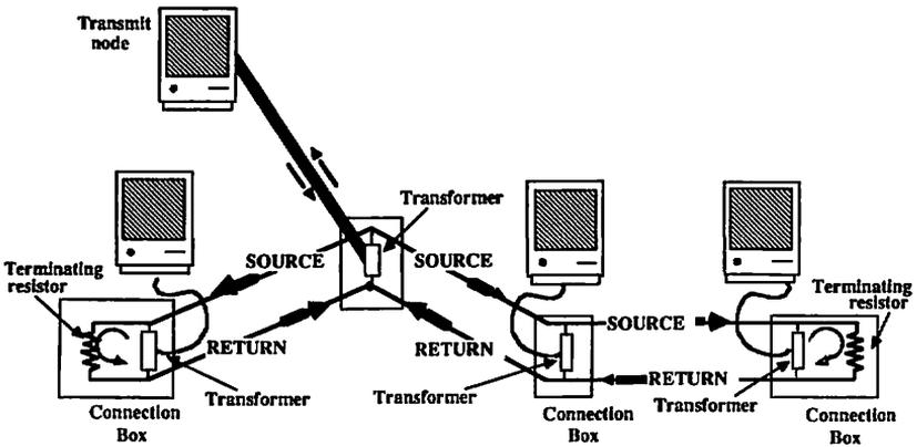
If the network cables are connected so as to form a closed loop, there is no way for the message signal on the source wire to flow to the return wire so the signals on both sides of the bus will collide with each other (shown below).
