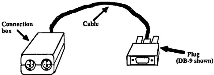
The **AppleTalk connector cable** permanently attaches the plug to the connection box. The plug for the Macintosh is a 9 pin DB type connector. For the Macintosh XL, the plug is a standard DB-25 connector.
