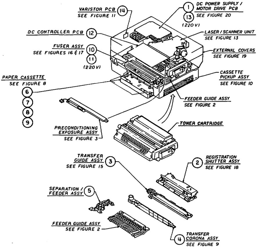
LASERWRITER - ASSEMBLY LOCATION DIAGRAMS (1 OF 2)
