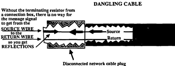
To prevent reflections of the message signal on the network, it is very important to always terminate the ends of the network cable into a connection box.
