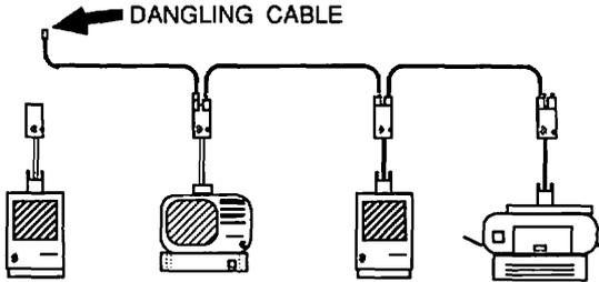
The message signal in a dangling cable has no place to flow once it reaches the end of the cable so it is reflected back on to the source wire, just like a flow of water run into a capped pipe (shown below).
