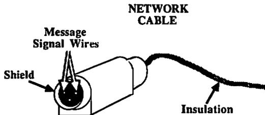
The two wires conduct the electric message signal to the AppleTalk connectors around the network.
