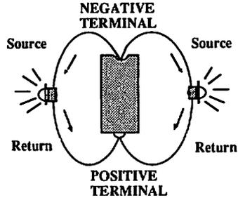
The current from the source (negative) wire flows through something called a load (a bulb for the flashlight and a terminating resistor for the AppleTalk bus) to the return (positive) wire. In the flashlight example above, two bulbs are shown to demonstrate that the current can be split at its source to travel through two loads and arrive at the same return point.
