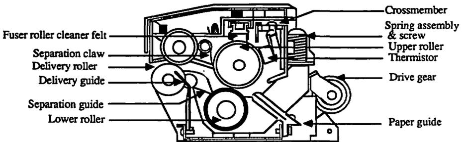
**CROSS SECTION OF FUSER ASSEMBLY**
