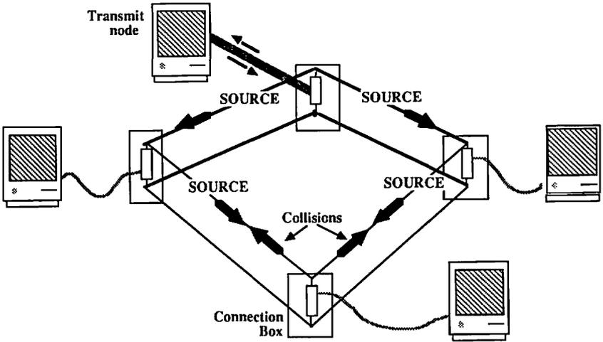
This would look like two nodes trying to talk at the same time, and that would interfere with communications. Therefore, it is very important to always terminate the ends of the network cable into connection boxes so that it does not form a closed loop.
