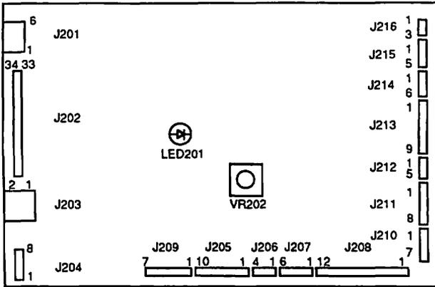
**FIGURE 3-3: CONNECTOR LOCATIONS ON THE DC CONTROLLER PCB**
