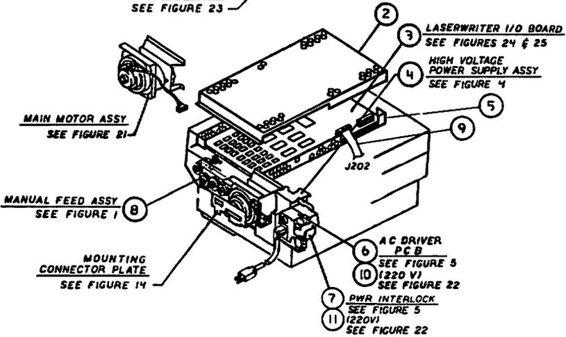
LASERWRITER - ASSEMBLY LOCATION DIAGRAMS (2 OF 2)
