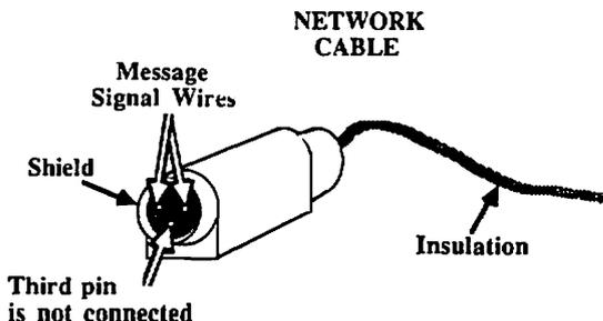
The two wires carry the message signals around the network.
