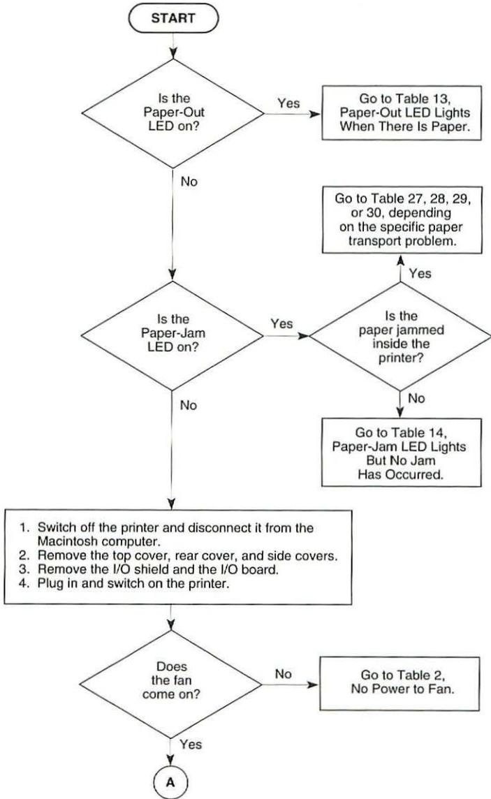
**Flowchart 4 LaserWriter Select 310 Print Engine Error (1 of 3)**
