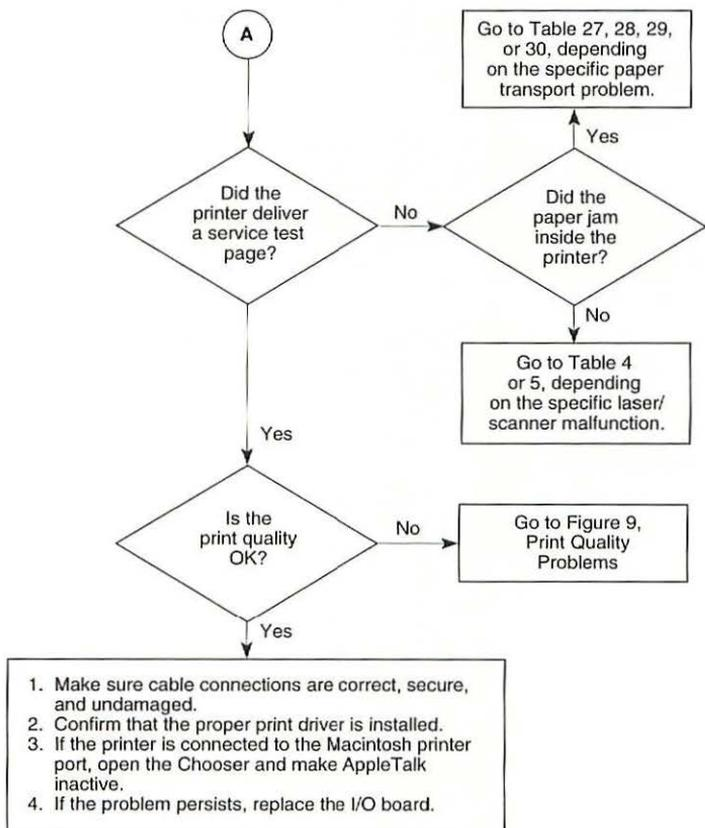
**Flowchart 2 LaserWriter Select 300 Print Engine Error (2 of 2)**
