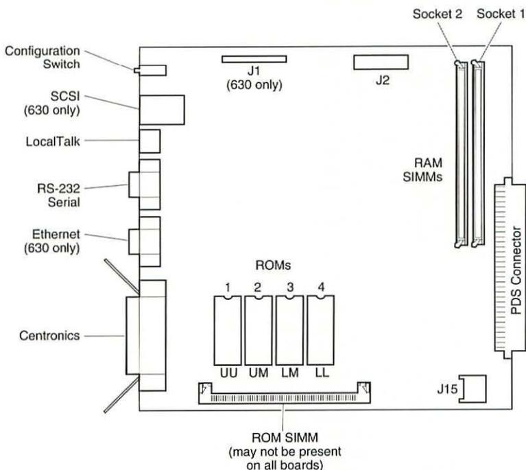
Figure 4 LaserWriter Pro 600 and 630 I/O Board
