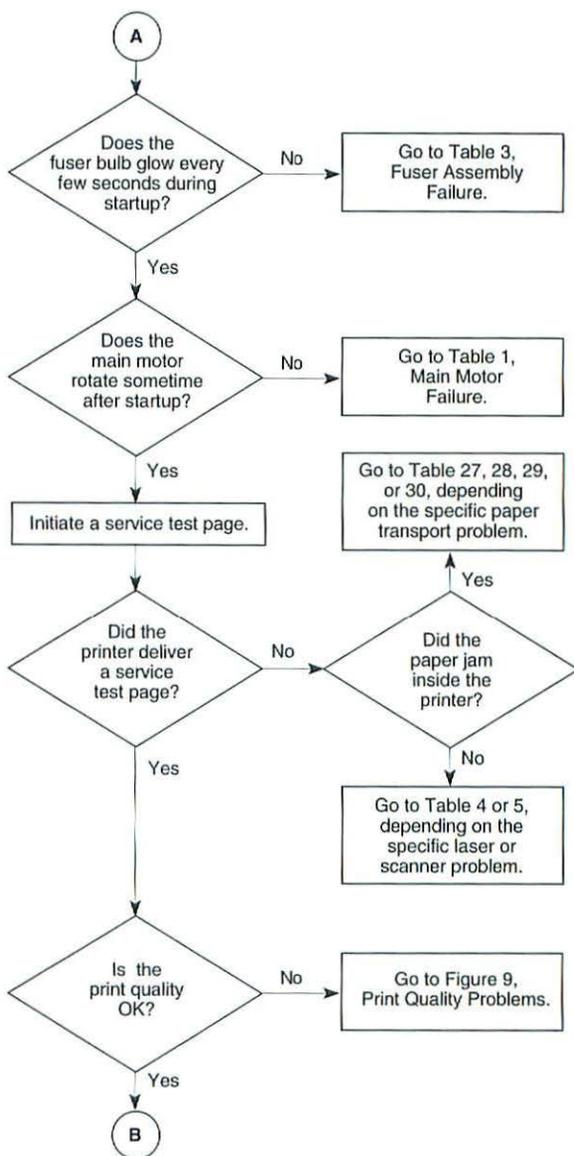
**Flowchart 4 LaserWriter Select 310 Print Engine Error (2 of 3)**
