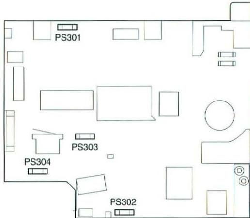
**Figure 7 Sensing System**
