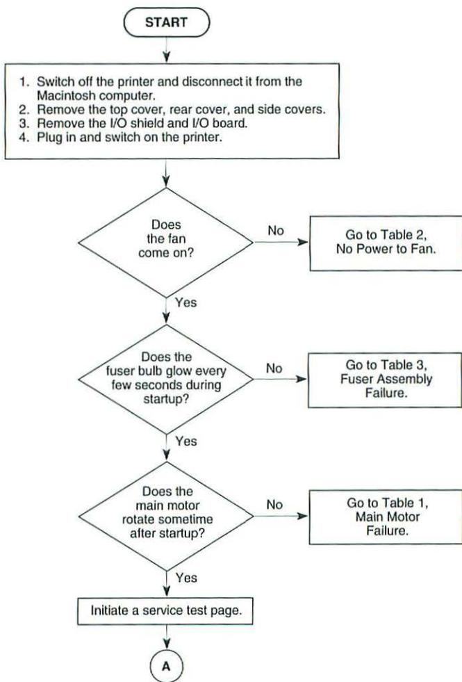
Flowchart 2 LaserWriter Select 300 Print Engine Error (1 of 2)
