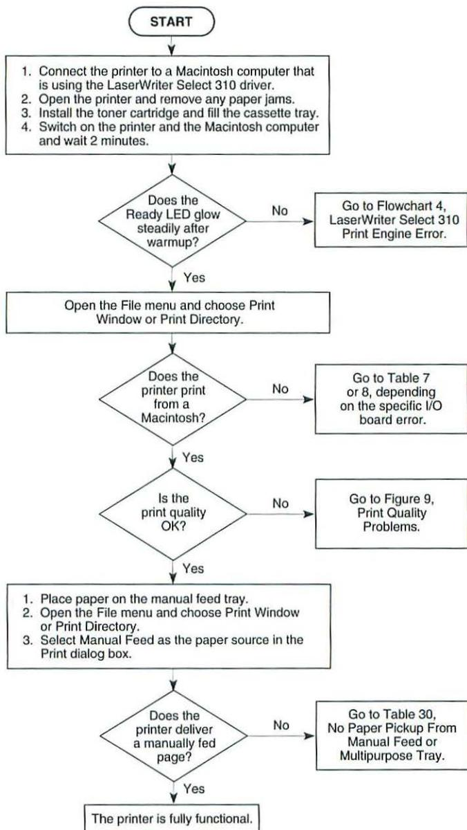
**Flowchart 3 LaserWriter Select 310 Print Engine Check**
