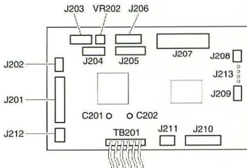
Figure 5 LaserWriter Pro 600 and 630 DC Controller Board
