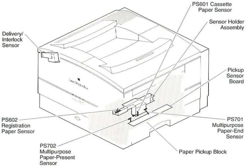
**Figure 11 Sensing System**
