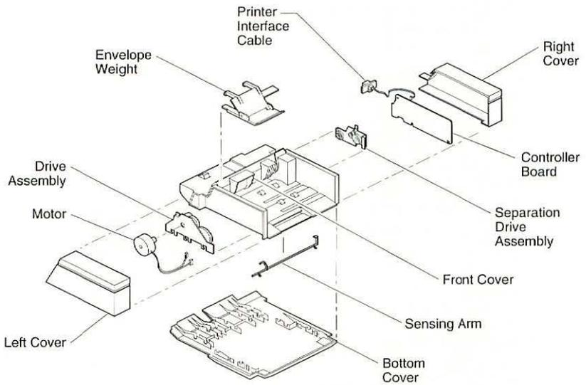
**Figure 2 LaserWriter Pro Envelope Feeder Exploded View**
