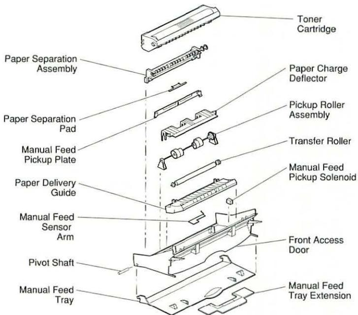
**Figure 1 LaserWriter Select 300/310 Exploded View (2 of 2)**
