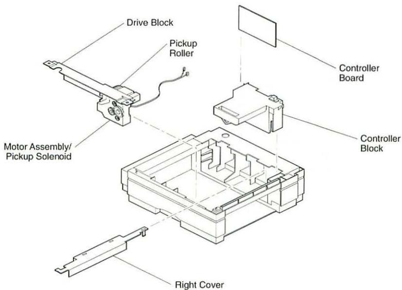
**Figure 3 LaserWriter Pro Sheet Feeder Exploded View**
