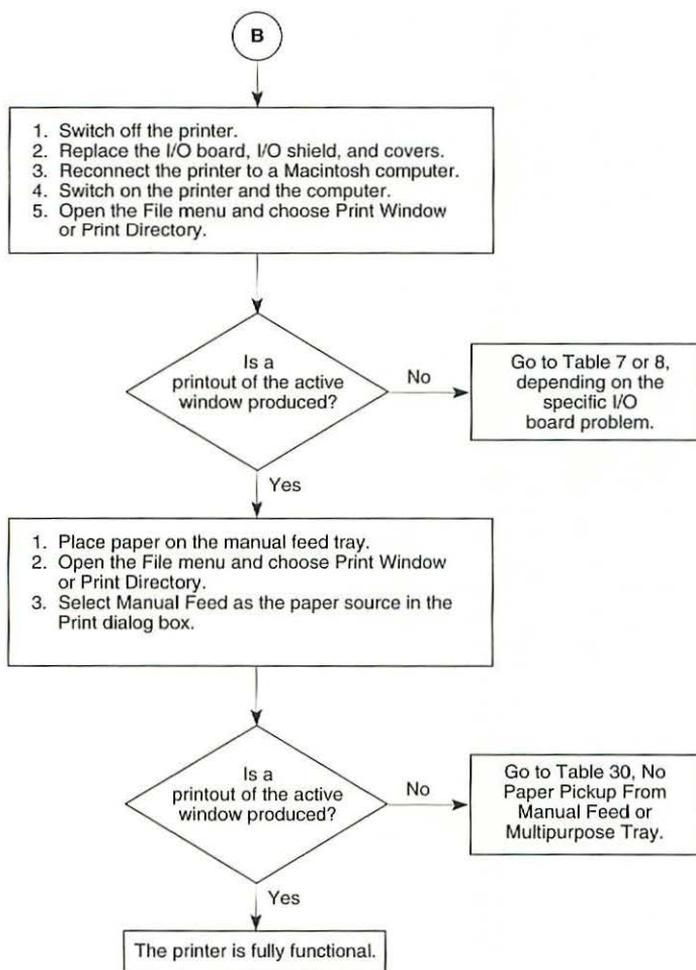
**Flowchart 4 LaserWriter Select 310 Print Engine Error (3 of 3)**
