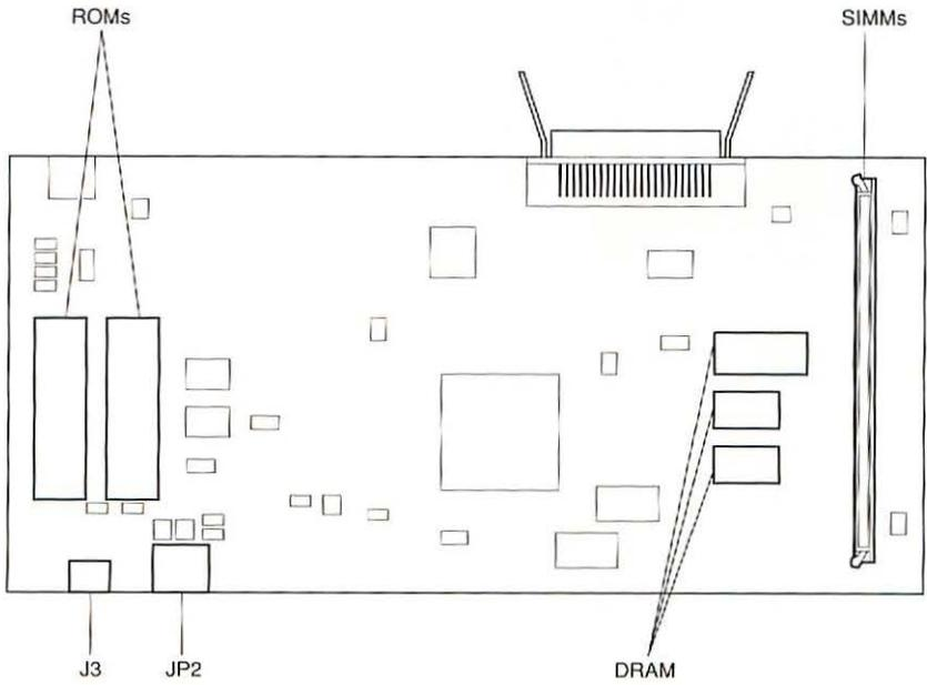
Figure 3 LaserWriter Select 310 I/O Board
