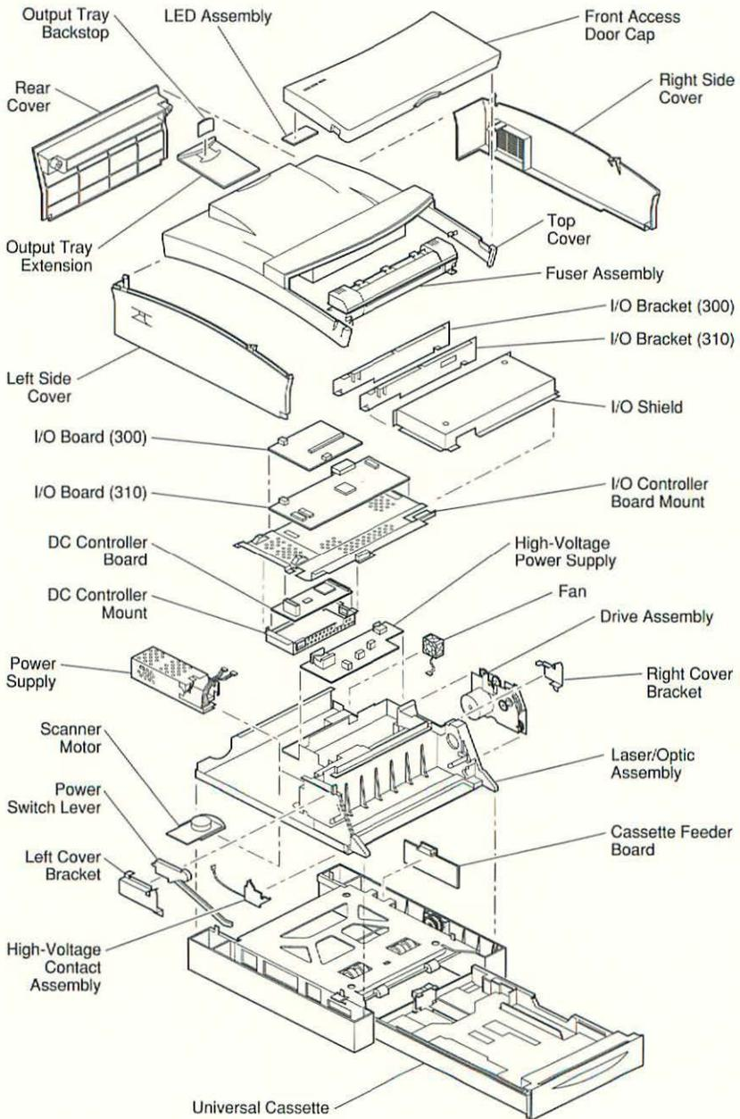
Figure 1 LaserWriter Select 300/310 Exploded View (1 of 2)
