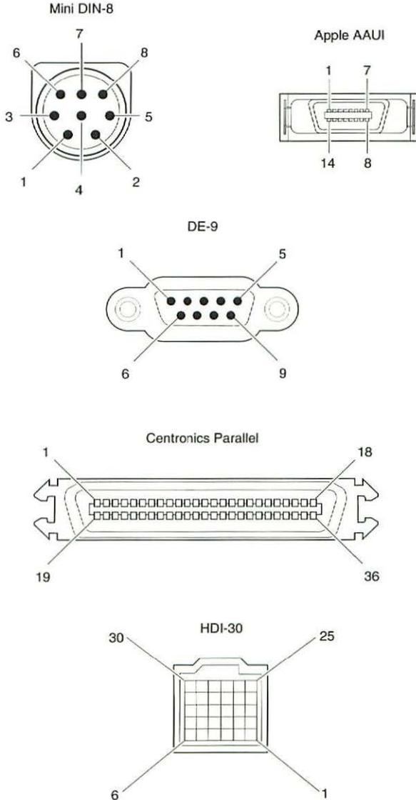
**Figure 3 Cable Connectors**
