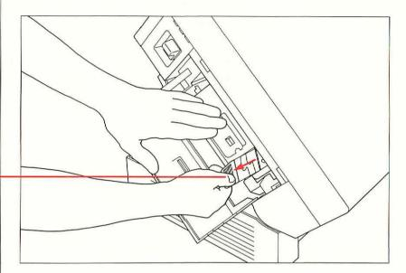
Pull out the tab and the attached tape
