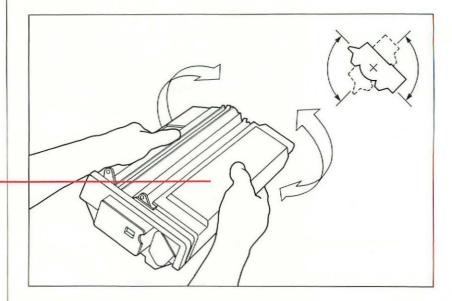
Open the upper unit of the LaserWriter by pulling up on the release lever, and then pull the cartridge door open.
