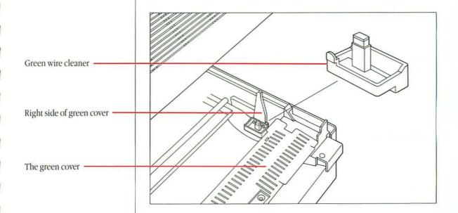
3. Lift the **green felt cover** and remove the **two orange cards** fitted into the cover's hinges.
