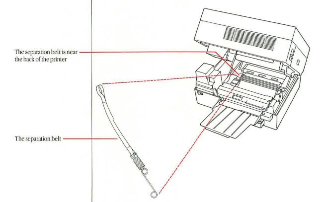
Follow the steps below and refer to the illustration to see how the separation belt should look when properly installed. If your final effort doesn't look like the illustration, pages won't feed correctly through the printer.
