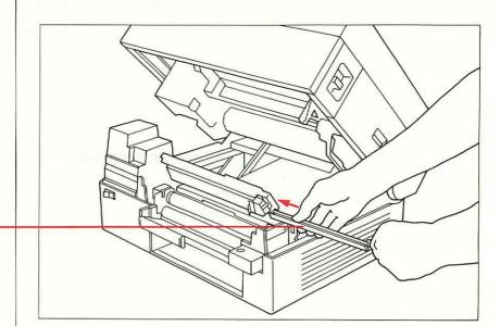
Remove the old and insert the new cleaning pad
