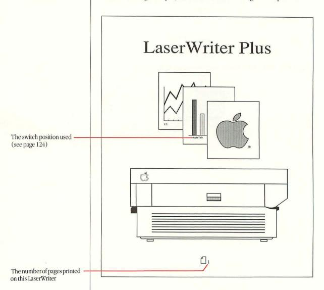
Sometimes the test page will be spotty because toner has spilled out onto the cartridge during shipment. If this happens, switch the LaserWriter off and on again to print another test page. Try this procedure two or three times; then if there's still a problem, refer to "Troubleshooting" in Chapter 4.
