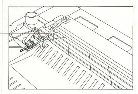
A properly installed separation belt
