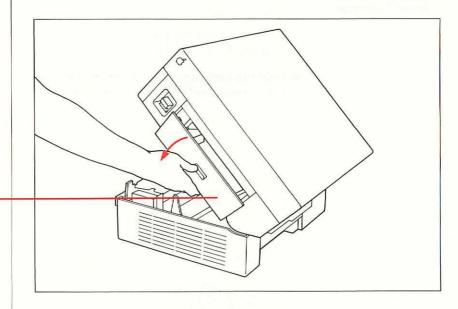
■ Slide the cartridge completely into the printer (the end with the small metal disk enters first) until you hear it click into place.
