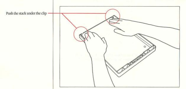
■ Slide the cassette into the lower slot on the same side of the printer as the paper output tray. The end with the clips enters first.
