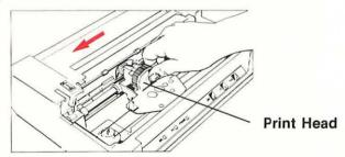
Replace the printer carrier cover by snapping it back into position. Your new printer is ready to be set up and tested.
