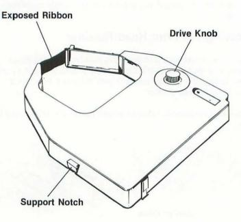
Remove the ribbon cassette from its wrapper. Turn the cassette drive knob in the direction of the arrow until the exposed ribbon is straight and taut across the cassette ribbon guides.
