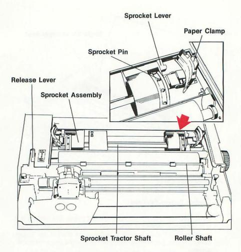
Open the two paper clamps. Fit the sprocket holes on the end of the paper onto the left sprocket pins, and close the paper clamp. Check to insure that the pin holes in the paper have set down over the sprocket pins. Follow these same steps, and load the paper on the right sprocket.
