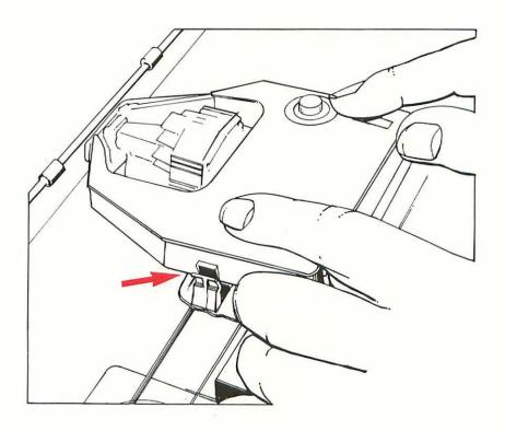
Turn the cassette drive knob clockwise until the ribbon slips completely into place. The drive knob is now engaged with the printer cassette drive gear. It will normally make a clicking noise as you turn it.
