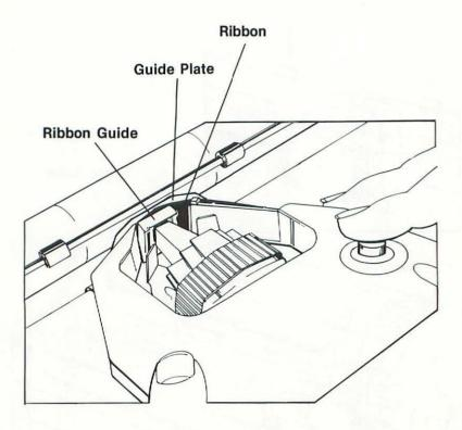
Using both hands, gently press the cassette down onto the ribbon deck until it snaps into place. Check that the two cassette locking tabs are holding the small notches on the sides of the cassette.
