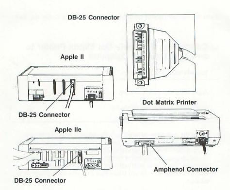
When connecting your printer to Apple II Series equipment you will only need to use the longer connecting cable from the DMP Connecting Cable Kit. Attach the DB-25 male connector on your printer connecting cable to the female receptacle on the Apple II Parallel Interface Card at the back of your computer cabinet. You should note that the connectors have a wide side and a narrow side. The matching sides of the connectors must be aligned before they will properly connect together.
