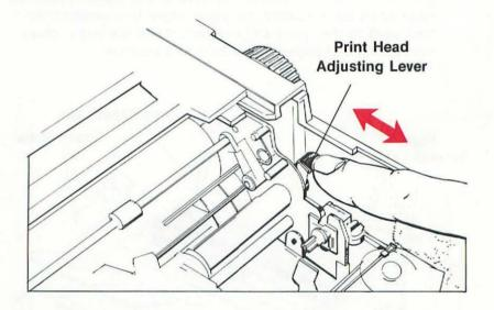
When the adjusting lever is pushed towards the rear of the printer, the print head is set for single-sheet printing.
