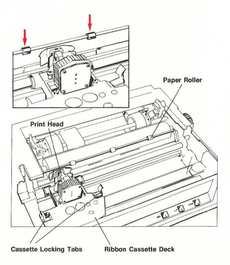
Holding the cassette in both hands and level with the ribbon cassette deck, carefully insert the exposed section of ribbon between the guide plate and ribbon guide. Make sure that the ribbon fits between these two parts.
