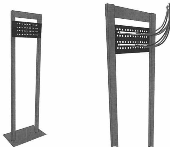
Front View of 72-Inch Rack with Patch Panel (left); Same Rack with Cables to 110-Blocks in Back (right)
