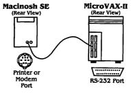
The Macintosh printer or modem ports, for example, can be connected directly to the VAX RS-232 ports with appropriate cabling. At the back of this booklet, the "Pinouts" appendix has more information on these ports.
