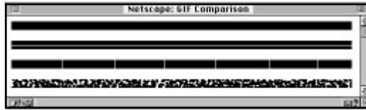
Figure 22.33 Four identically sized and created GIF images take up different amounts of disk space.
