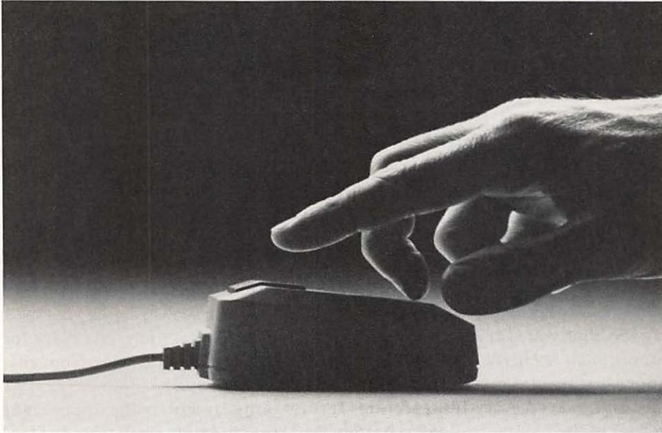
**Fig. 1-6** Instead of keyboard-entered commands, most operations depend upon pointer selections made by movement of the mouse. A single button directs entries.
