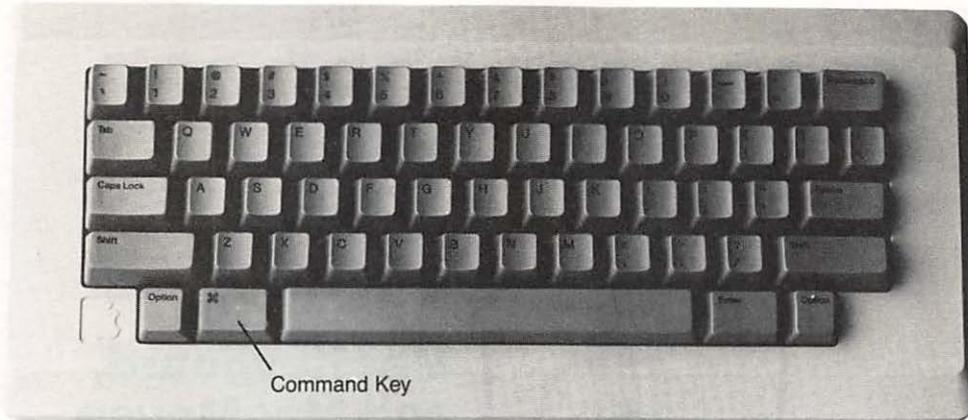
**Fig. 3-1.** In all, 256 different characters can be entered from the keyboard. Note the **OPTION**, **ENTER**, and **BACKSPACE** and command keys.
