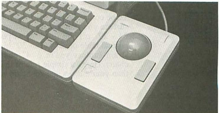
Another kind of alternate input device is the mouse substitute. Usually a ball you spin or a disk you push down the edges of, it sits next to the keyboard (much as a numeric keypad does) and lets you move the pointer around the screen with your fingers instead of your arm. The makers of some mouse substitutes claim that they're faster, more accurate and easier to use than a mouse; at the very least, they cut down on how much physical work you have to do.
