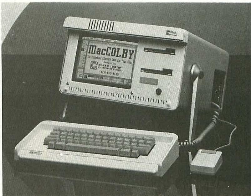
This repackaged Mac has a fan, and there's also room in the box for a second disk drive (or a hard disk), a video output board (for driving external monitors), a DC converter (so you can run it off your car battery) and a modem. You can buy it two different ways—all put together (for about \$500 more than an equivalent Mac in the standard configuration), or as a conversion module that lets you convert a conventional Mac to a MacColby.
