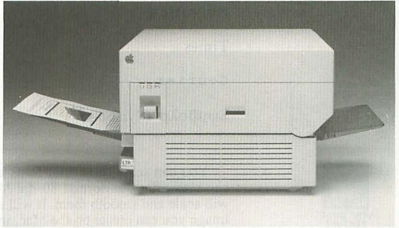
Like most inexpensive laser printers, the LaserWriter is built around the Canon LBP-CX "engine" (mechanism). To this basic engine, Apple has added 1.5 *megabytes* (1536K) of RAM, 512K of ROM, a 68000 chip just like the one in the Mac (except this one runs 50% faster), and an interface to **AppleTalk**, Apple's "local area network" that links computers and peripherals together.
