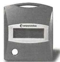
The Canary Wireless Digital HotSpotter shows the network name, signal strength, channel, and open/closed status.
