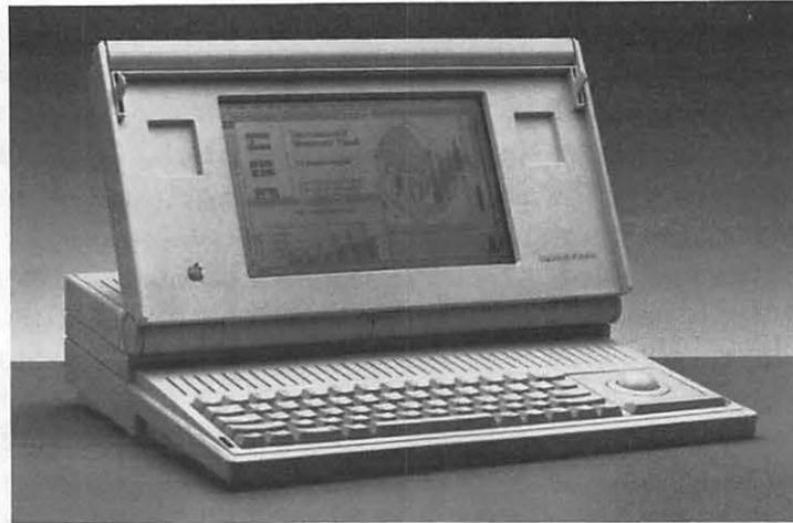
The Portable has a power manager chip to conserve battery life. It comes with one megabyte of RAM, and a 40-megabyte hard disk is available as an option.
