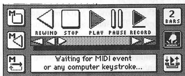
So how does a sequencer know when to start and stop? Start, stop, and continue messages are responsible for functions that, if they controlled a tape recorder, would include play/record, stop, and rewind. The *start* signal begins playing or recording a sequence from its beginning. I surely don't need to tell you what *stop* does.
