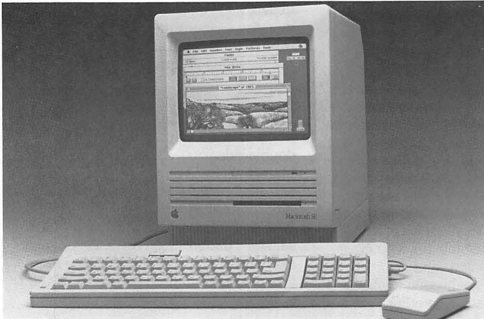
The SE is available with two internal floppy drives or with an internal hard disk and a single floppy drive. Newer SEs contain Apple's 1.4-megabyte (1400K) FDHD drive which reads and writes to disks formatted for the Mac, MS-DOS, OS/2, and ProDOS.
