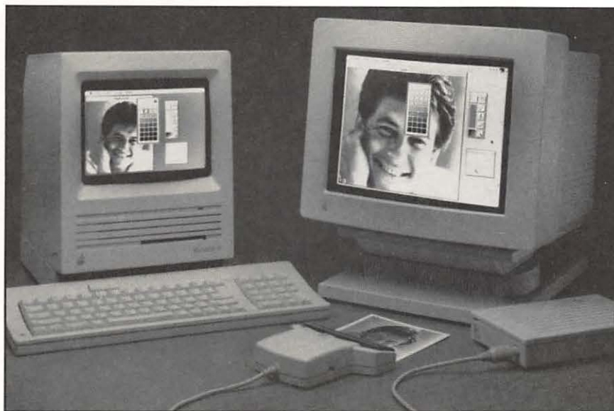
A ScanMan hand-held scanner by Logitech for the Macintosh Plus, SE and II. Hand-held scanners are inexpensive, easy to use, and provide a quick way of scanning small pieces of artwork.
