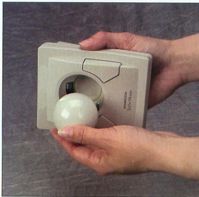
*Removing the roller ball from the trackball.*
