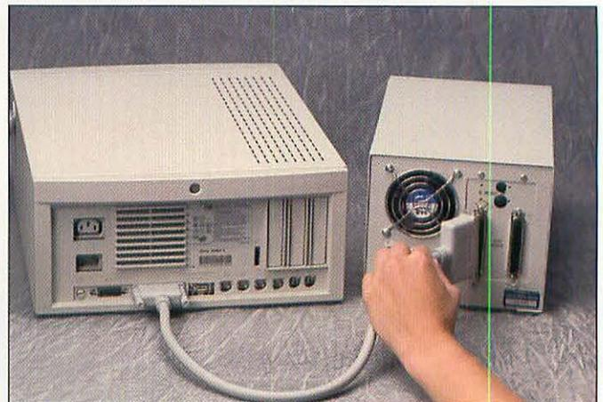
*Hooking the SCSI cable to the hard drive.*
