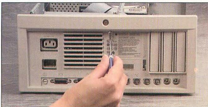
*Removing the power supply screw.*
