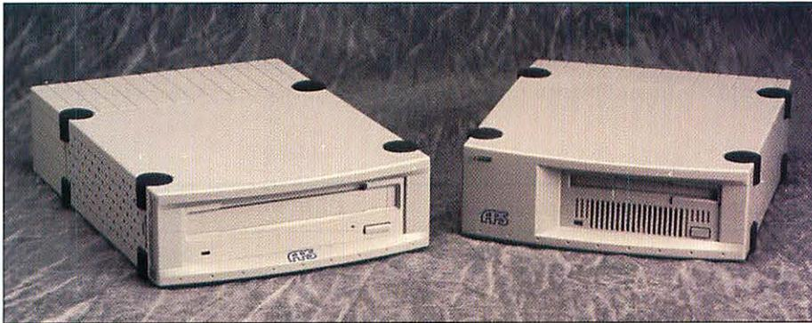
*A 1.3-Gb magneto-optical drive (left) and a 128 Mb drive (right).*
