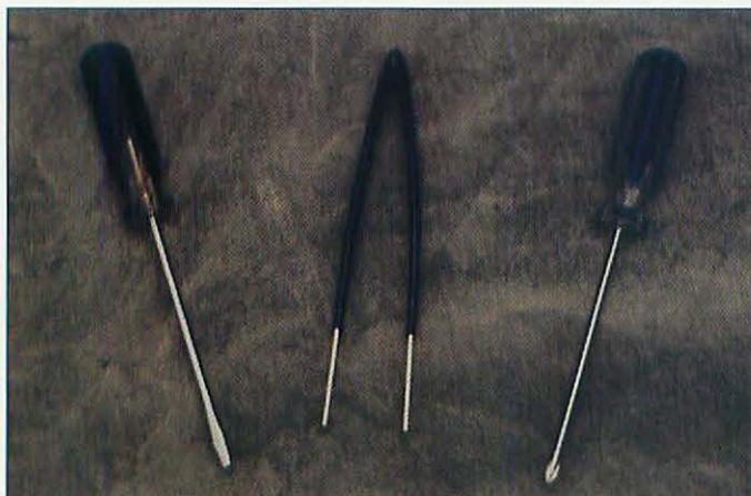
*A flat-blade screwdriver, tweezers, and a Phillips screwdriver.*
