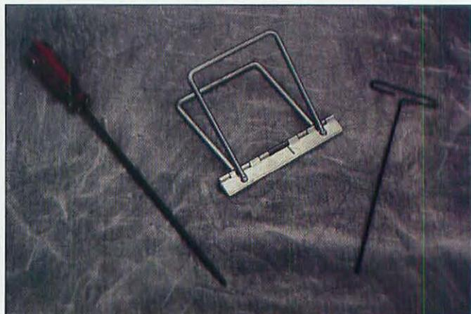
*The Mac Cracking kit (for compact Macs only). The Torx T-15 screwdriver is on the left; the case spreader is in the middle. The tool on the right is a less-expensive version of the Torx screwdriver.*
