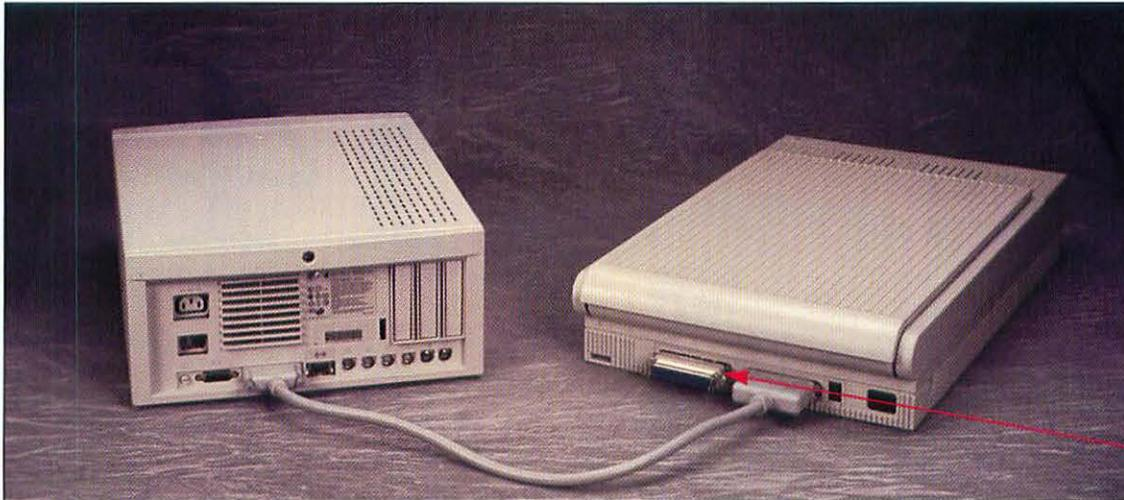
The SCSI cable and terminator on the scanner.
