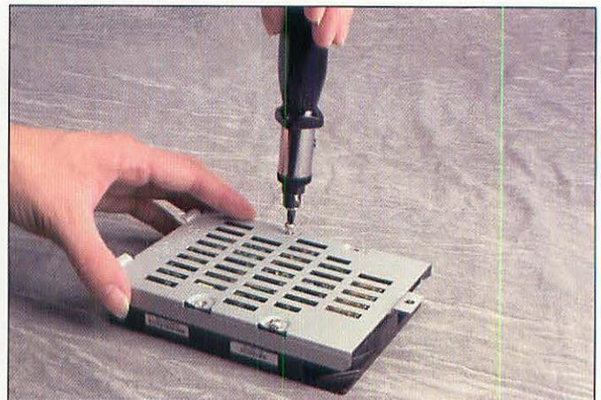
*Attaching the bracket to the new drive.*
