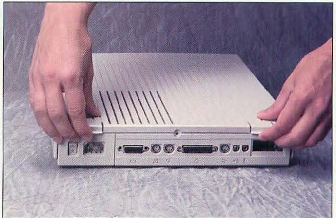
Lifting the case release latches.
