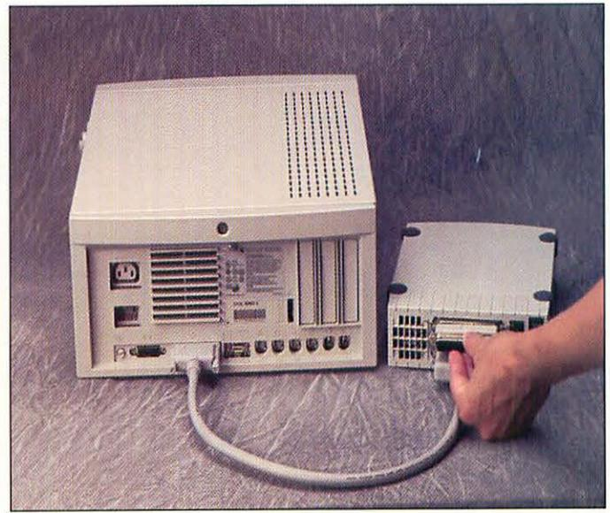
*The SCSI cable and terminator on the tape drive.*
