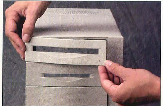
Snapping the new bezel into place.
