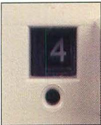
*Two other types of SCSI ID selectors. To change the one on the top, insert a small tool in the hole and press to make it click. Change the one on the bottom by turning the dial with a small screwdriver.*
