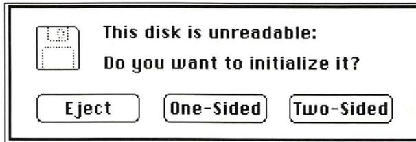
Normally, you'll initialize both sides of a two-sided disk to take advantage of increased speed and capacity, and the hierarchical file system. A disk initialized double-sided lets you use folders within an application as well as in the Finder. The Apple 3.5 Drive uses both sides of the disk, giving you 800K of storage on a disk initialized double-sided.
