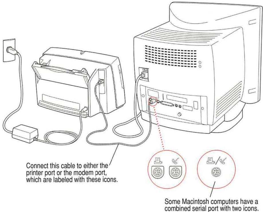
If your computer is connected to a network, a network cable may already be connected to the printer port (🖨️). In that case, use the modem port (📞).
