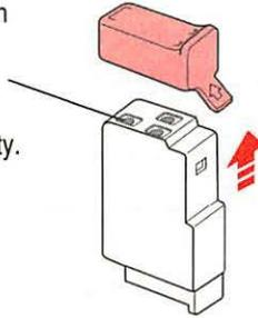
**6** Slide the tank into the cartridge, and push it down so it snaps into place.
