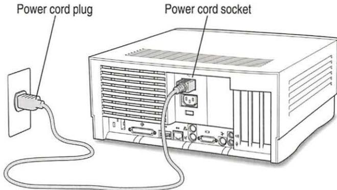
**IMPORTANT** The only way to disconnect power completely is to unplug the power cord. Make sure that at least one end of the power cord is within easy reach so that you can unplug the computer when you need to.
