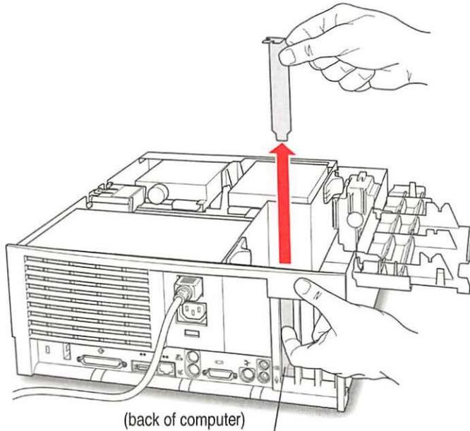
Push the port access cover in gently with the finger of one hand while pulling it straight up with the other hand.
