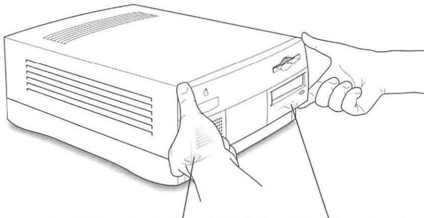
Locate the two release buttons under the front panel ledge with your fingertips.
