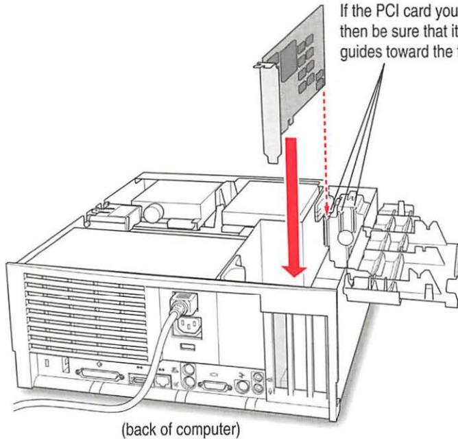
**9 Press the card gently but firmly until the connector is fully inserted.**
