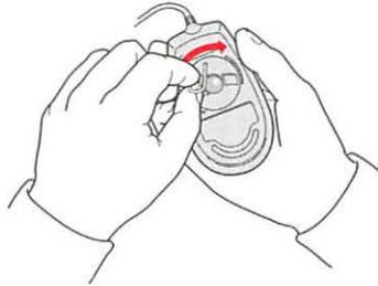
Turn the ring a very short distance, until it stops. When the recessed area on the ring is *not* lined up with the recessed area surrounding the ring, the mouse is locked.
