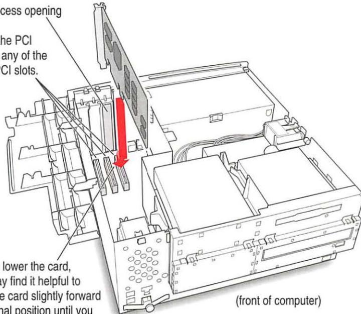
If the PCI card you are installing is full-length, then be sure that it fits in one of the three card guides toward the front of the computer.
