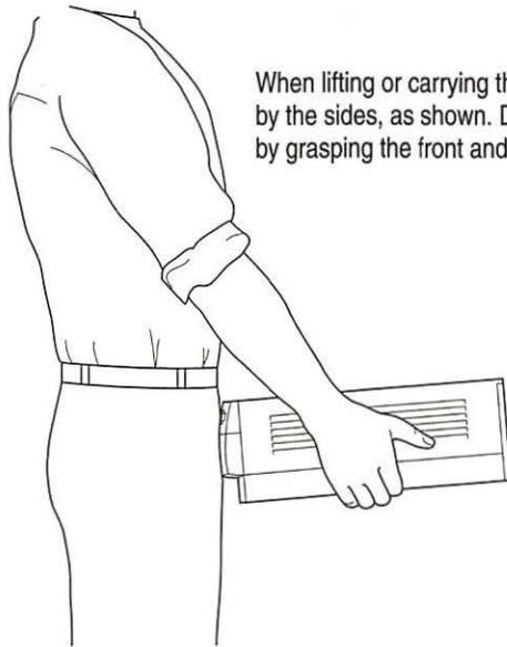
When lifting or carrying the computer, always grasp it by the sides, as shown. Do not lift or carry the computer by grasping the front and back.
