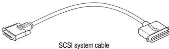
If the device is not the first one, use a SCSI peripheral interface cable to connect it to the last device in the chain:
