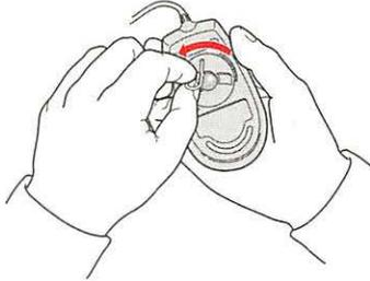
Turn the ring a very short distance. When the recessed area on the ring is lined up with the recessed area surrounding the ring, the mouse is unlocked.
