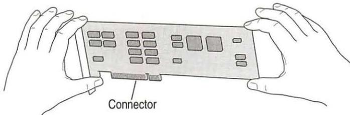
**8** Align the connector end of the card with the expansion slot.
