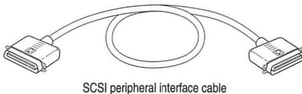
**IMPORTANT** The total length of the cables in a SCSI chain should not exceed 6 meters (20 feet). SCSI cables must have a 110-ohm impedance. For best results, use SCSI cables manufactured by Apple Computer.
