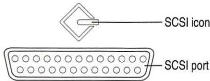
You can connect SCSI devices to the SCSI port in a chain. The first device in the chain plugs into the SCSI port; the second device plugs into the first device, and so on. SCSI devices commonly used with the Macintosh include hard disk drives, CD-ROM drives, scanners, printers, and tape or cartridge backup drives.
