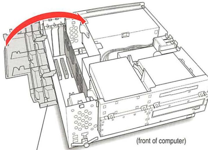
Flip the expansion card cover closed and snap it into place.
