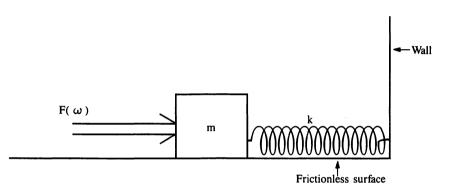
If the weight is subject to a driving force  $F \sin(\omega t)$  ( $\omega$  represents the frequency of the driving force and t is time), the equation of motion of the mass is as follows:
