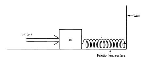
If the mass is subject to a driving force  $F \sin(\omega t)$  ( $\omega$  represents the frequency of the driving force and t is time), the equation of motion of the mass is as follows:
