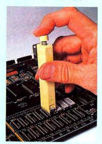
Install the PC board. This houses the enclosed multiplexer.
