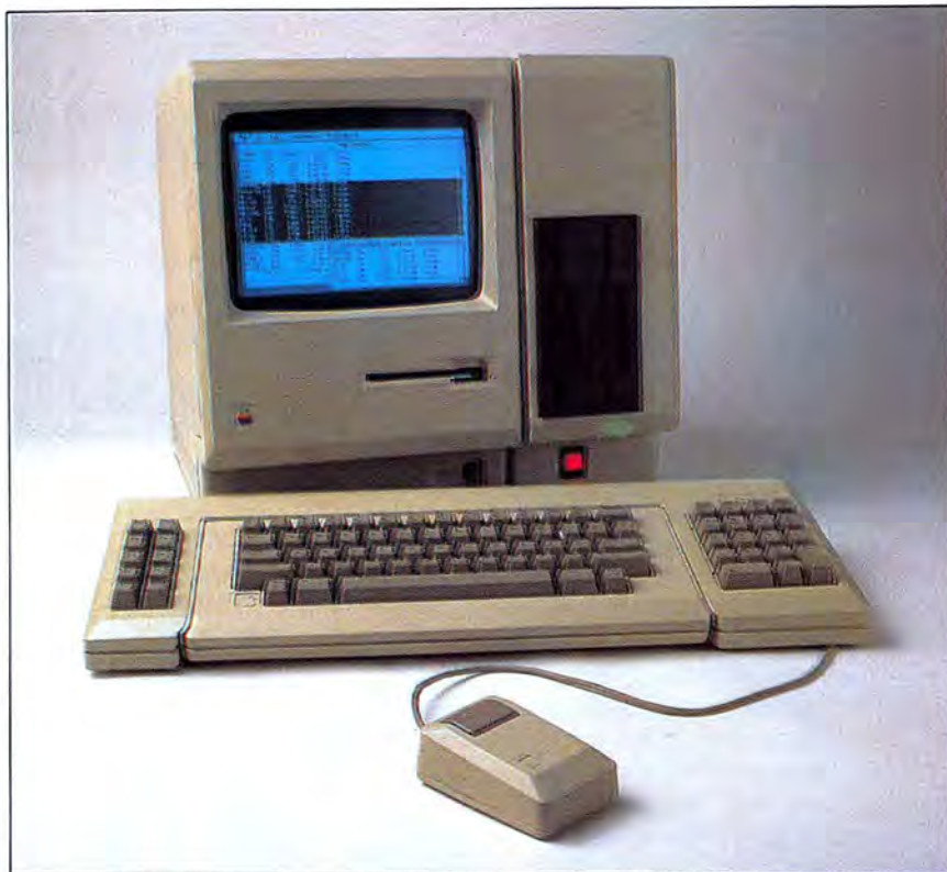
MacCharlie piggybacks off the Mac monitor and keyboard. The Mac desktop, including desk accessories and Clipboard are always present behind MS-DOS.
