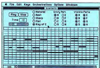
Fig. 2: Music is entered into StudioMac through proportional notation. The bass and cleff staves stand out from the background grid, and the user "draws" notes onto the grid. The different colors denote the discrete voices.
