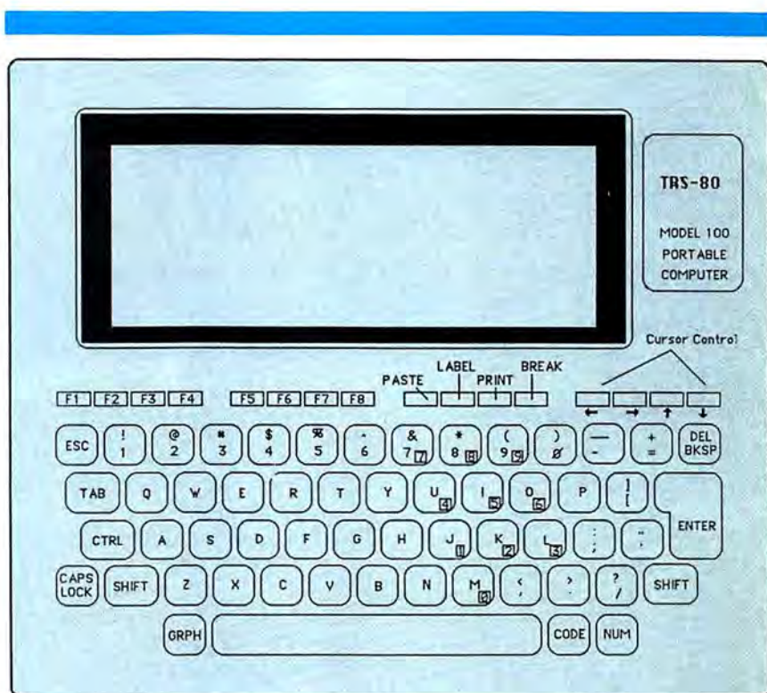
Fig. 1: The TRS-80 Model 100 keyboard. There are eight software defined function keys, F1-F8. Their functions vary depending on the program in use. In addition there are four predefined function keys: PASTE, LABEL, PRINT and PAUSE/BREAK. The PASTE key takes any material cut or copied into the paste buffer and pastes it into the current document. Pressing LABEL displays the functions attached to function keys 1-8 across the bottom of the screen. PRINT sends a
