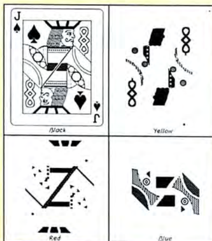
The figure has to be divided into images for each of the colors to be printed. Note the solid block for the Jack's hair in the yellow image, which will be overlaid with the black curls; all of the yellow images are framed in another color so they will show up better.
