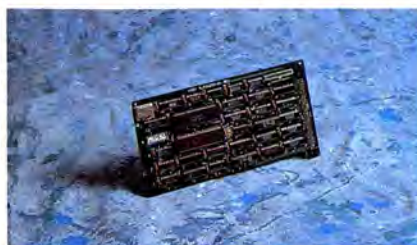
The AST Mac86 is an 8086-based coprocessor board that enables users to run MS-DOS application software on the Macintosh SE as well as moved back and forth between the two environments.
