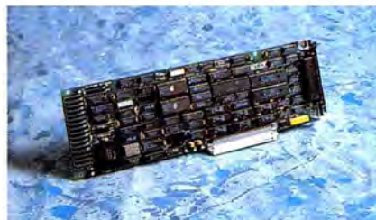
The AST-ICP is an intelligent communications processor that offloads communications functions from the Macintosh II to increase system performance, speed and efficiency.
