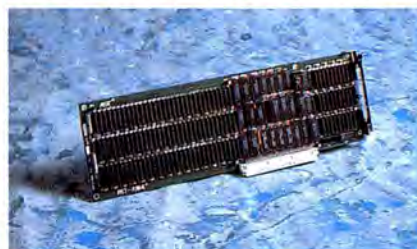
Designed to complement the Macintosh II computer, the AST-RM4 memory expansion board provides up to four additional megabytes of memory.
