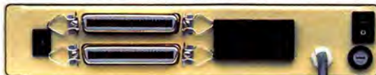
Our original SCSI select switch allows you to add another drive or tape backup with one push of a button. No longer do you have to open up a box to assign the SCSI port number.
