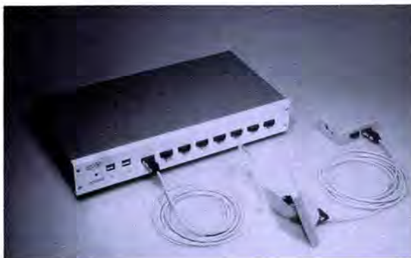
Key components of Du Pont's fiber optic local area network are, (from L to R), the concentrator, wall plate and converter.
