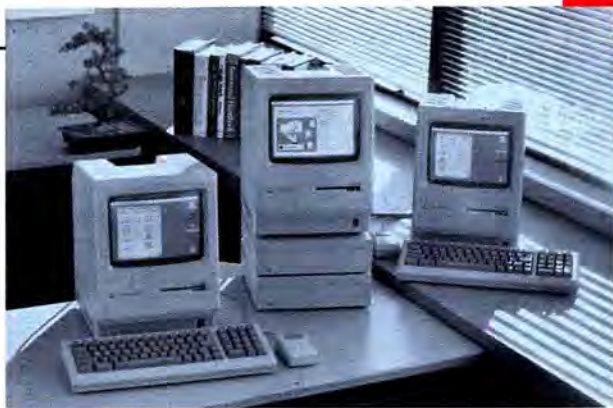
The AppleShare file server configuration is flexible and expandable — consisting of a Macintosh Plus with virtually any hard disk.
