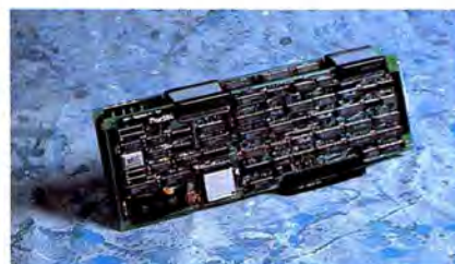
The AST Mac286 is an 80286-based microcomputer that allows a user to run MS-DOS applications at IBM PC AT speeds on the Macintosh II computer.
