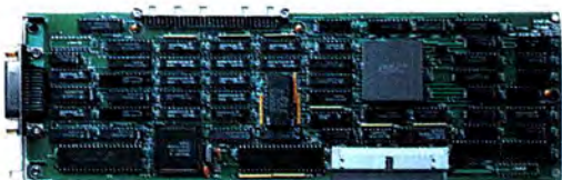
In scientific or engineering applications, a special card can connect an SE or a II to lab instruments.
