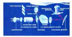
Videodiscs store data as a series of pits. A laser beam reflecting off of the pitted surface results in a modulated signal that is then converted into an electrical composite audio/video signal.
