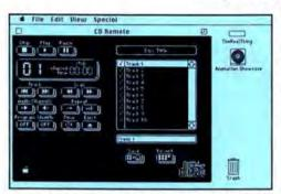
Apple's CD Remote desk accessory is difficult to read on-screen, but it lets you program and replay tracks on its CD SC optical-disc drive. The drive reads discs containing up to 656 megabytes of information and plays regular audio CDs as well.
