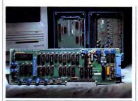
Data? You need data? GW Instruments has just released the MacADIOS II Jr, a low-cost addition to its MacADIOS line of data-acquisition boards. Mac SE owners can use this Mac II board with an optional expansion kit.
