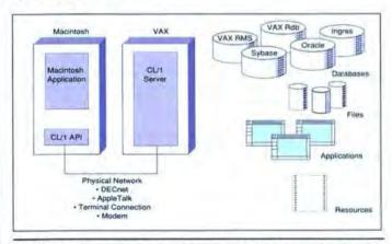
Figure 2: CL/1 will connect Macs to many VAX databases. The Macintosh communicates with a CL/1 Application Programming Interface (API), which sends the requests to a CL/1 server on the VAX.
