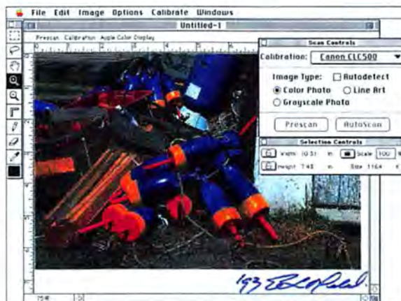
The new color version of Ofoto provides a set of built-in calibrations for many desktop color printers and for most popular laser printers. Ofoto not only automatically cropped the image shown here but was smart enough to include the photographer's signature in the crop area.
