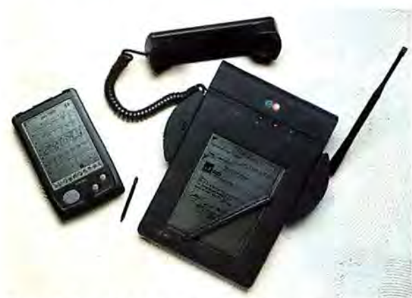
Figure 5: Due this fall, the Zoomer (left) is a $699 organizer that will be manufactured by both Casio and Tandy. The Zoomer is the same size as the MessagePad and sports many of the same features. The AT&T EO Personal Communicator (right) is larger and heavier than the MessagePad but offers more storage options, a higher-speed fax modem, and a cellular phone.
