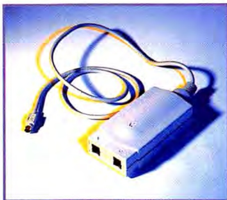
Figure 1: The GeoPort Telecom Adapter — the phone pod — is a line adapter that converts incoming and outgoing telephone signals into the format appropriate for your AV Mac and the phone system to which it's connected.
