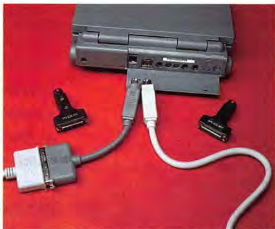
figure 1 / The PowerBook's special HDI-30 SCSI connector requires a special SCSI cable. The platinum-colored Apple HDI-30 System Cable is for attaching an external SCSI device to your PowerBook. The shorter, dark-gray Apple HDI-30 SCSI Disk Adapter is for using the PowerBook as a SCSI drive. If you don't want to mess with special cables, get an adapter such as the APS SCSI Boy or SCSI Doc, each of which can provide the PowerBook with a standard, desktop-Mac SCSI connector that attaches to a standard SCSI system cable. Both APS adapters let you connect the PowerBook to SCSI devices; the SCSI Doc also lets you use the PowerBook as a SCSI device.
