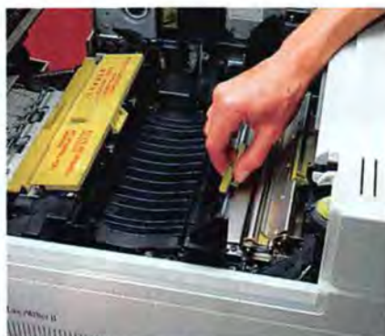
figure 1 / Dried toner on your printer's corona wire blocks portions of an image from printing. To clean the wire, use the printer's cleaning tool — or a cotton swab and isopropyl alcohol.
