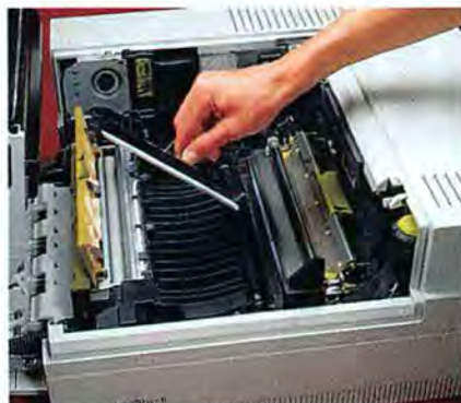
figure 2 / Replacing the fuser wand, usually located on top of a printer's fuser rollers, can solve the problem of unwanted dots, stains, and lines on the printed page.
