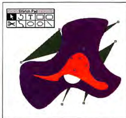
figure 3 / SXetch Pad brings some of the power of a draw program to QuarkXPress, adding Bézier-curve tools and multicolor blends.
