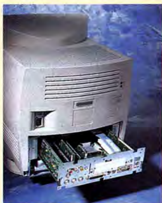
Accessing the motherboard is as easy as sliding open a desk drawer.
