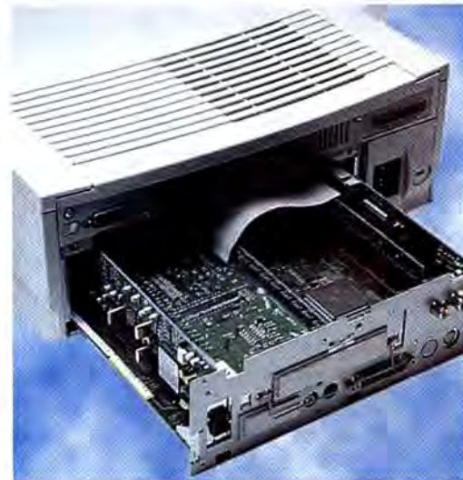
figure 1 / To use an external modem with the Performa 6200CD, remove the internal-modem card (at right) and then pop out the plastic plug on the back of the machine.
