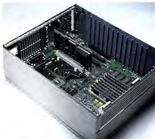
figure 2 / This two-tiered accelerator board replaces the Ilcx's original 68030 processor with a relatively speedy 68040.
