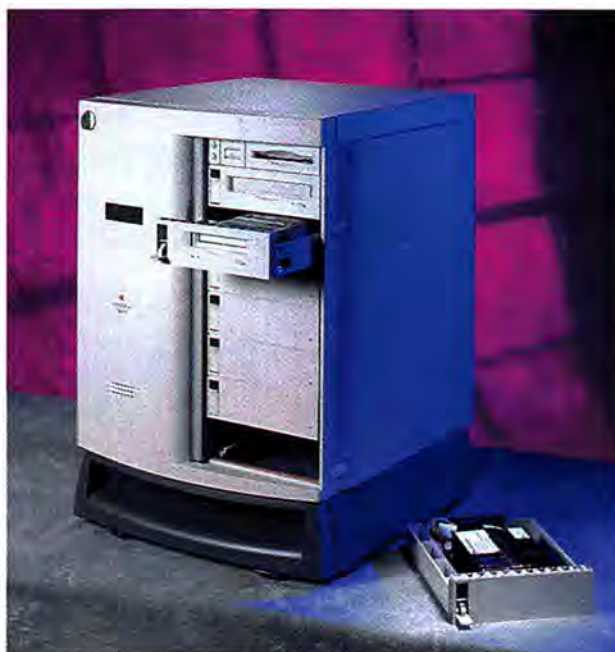
Apple's Network Server cabinet design is completely modular, with fully hot-swappable components.
