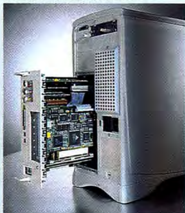
A slide-out logic board makes for easy upgrading.
