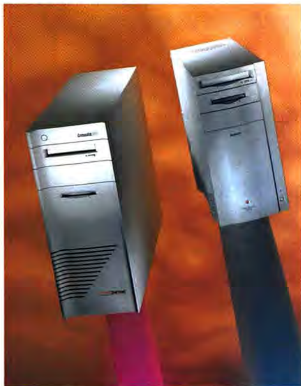
Twin-powered towers , the DayStar Genesis MP 360+ and the Apple Power Mac 9500/180MP both feature dual 180-MHz PowerPC 604e processors.
