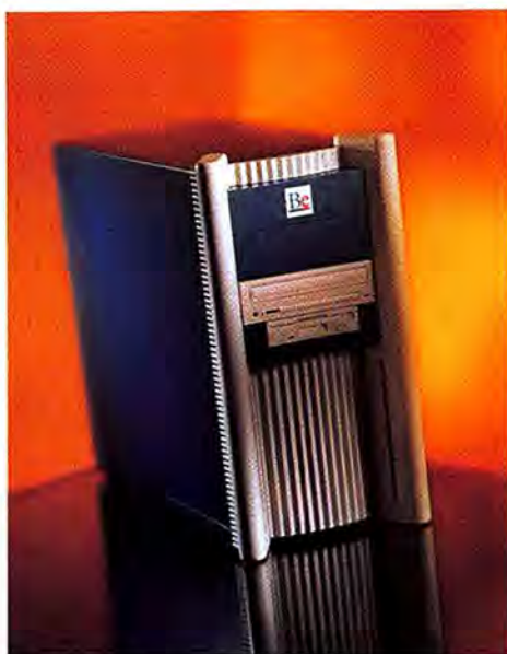
The BeBox offers two PowerPC processors and a plethora of ports for under $3,000.
