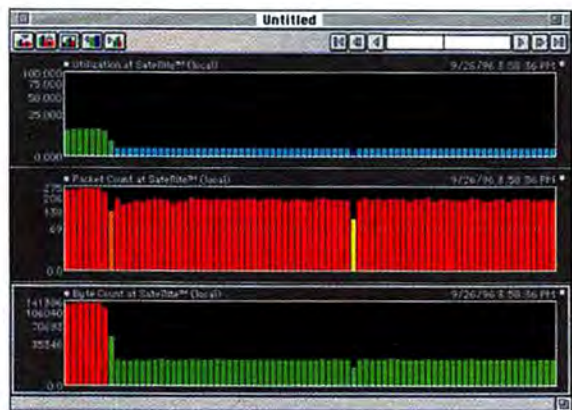
figure 1 / The AG Group's Skyline tool enables you to gauge whether your network is overutilized. If network traffic resembles that shown here, chances are that the problem lies with the server, not the network.
