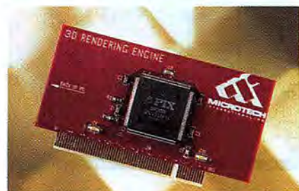
Because its 5-MOS PIX 3-D-graphics-accelerator chip has its own built-in PCI interface, the Microtech 3D Xplosion is the least crowded PCI card we've ever seen.
