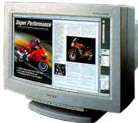
The vast 1,920-x-1,200-pixel screen of the Sony Multiscan GDM-W900 fits two WYSIWYG pages, with plenty of room for palettes.
