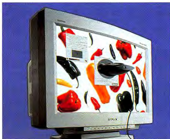
The Light Source Colortron II spectrophotometer and its powerful software (both bundled with the Sony Multiscan GDM-W900) enable the compact unit to function not only as a precision monitor calibrator but also as a handheld color-measurement and -specification device, usable on a wide variety of reflective surfaces.
