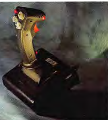
Figure 1 • The more buttons the better. If you're playing a complex Mac flight-simulator game, a joystick such as this button-studded F-16 Fighterstick, from CH Products, is crucial.
