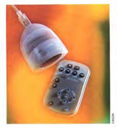
Mac's USB port. The remote provides typical controls—including play, pause, reverse, fast-forward, volume up, and volume down —as well as a button that lets you cycle through open applications.
