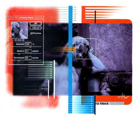
The Unsharp Mask filter (Filter: Sharpen) compares each pixel in your image to its neighboring pixels; the greater the contrast between two pixels, the more the program increases the contrast. This results in a halo effect around edges that appears to increase an image's sharpness (see the sidebar "Behind the Unsharp Mask Filter").
